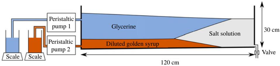
FIGURE 1. Experimental set-up.
