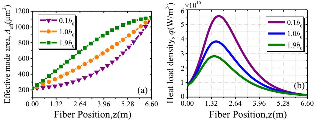
**Figure 9.** (a) Effective mode area of LP<sub>01</sub> and (b) heat load density evolution along T-SCF.
