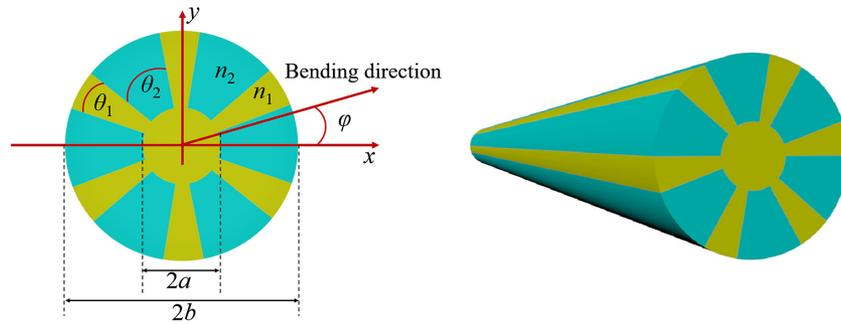
Figure 1. Schematic diagram of the SCF,  $N = 6$ <sup>[25]</sup>.
