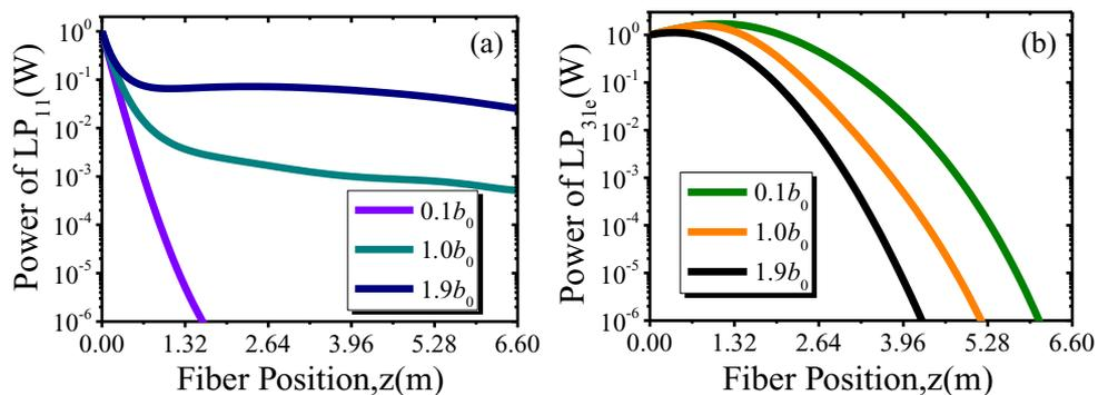
**Figure 11.** Power evolution of (a) LP<sub>11</sub> mode and (b) LP<sub>31e</sub> mode in the T-SCF under a bending radius of 32 cm.
