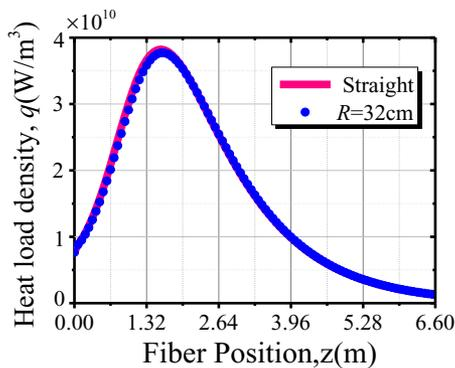
**Figure 12.** Comparison of heat load density between straight T-SCF and bent T-SCF of  $R = 32$  cm.
