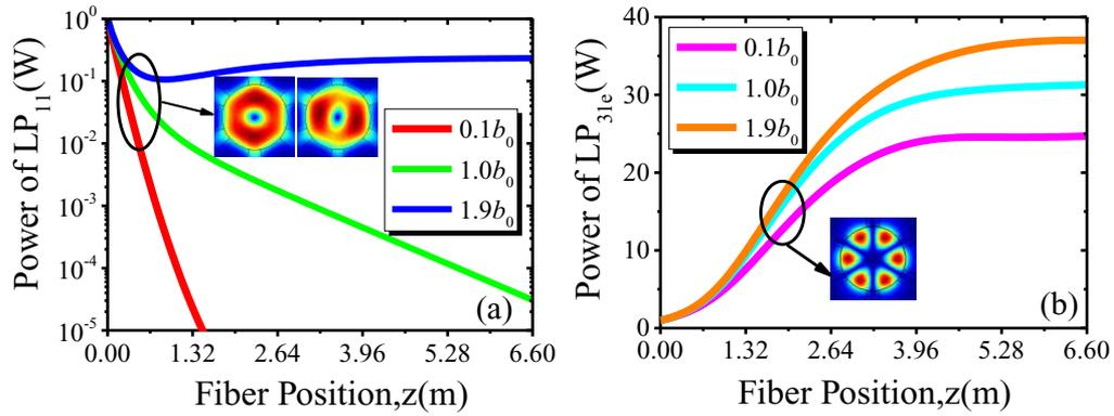
**Figure 8.** Modal power evolution of (a) LP<sub>11</sub> mode and (b) LP<sub>31e</sub> mode for concave, linear, and convex T-SCF based on the small-to-large amplification scheme.
