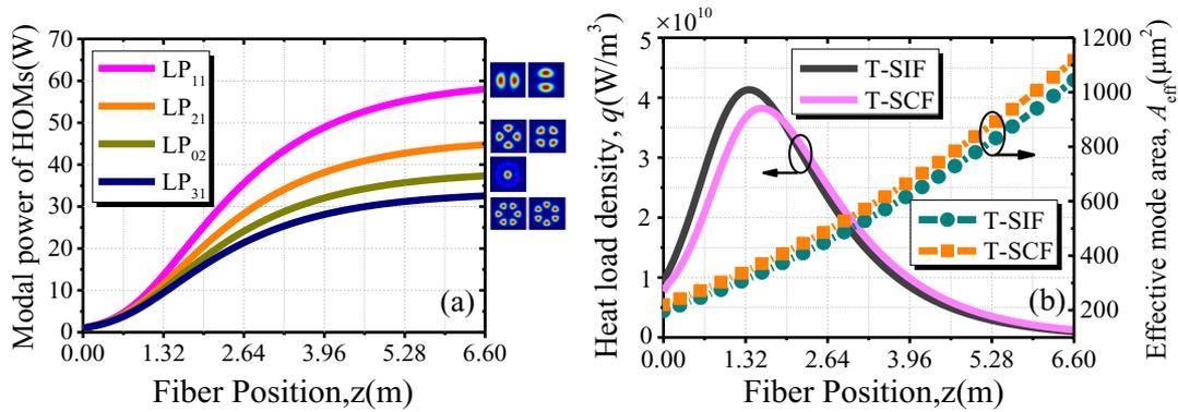
**Figure 10.** (a) Modal power evolution of four HOMs in linear T-SIF and (b) comparison of heat load density and effective mode area of LP<sub>01</sub> between linear T-SCF and T-SIF.
