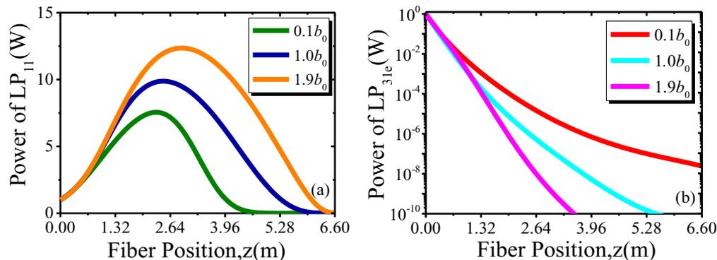
Figure 16. Power of (a) LP<sub>11</sub> and (b) LP<sub>31e</sub> of the T-SCF under a bending radius of 32 cm.
