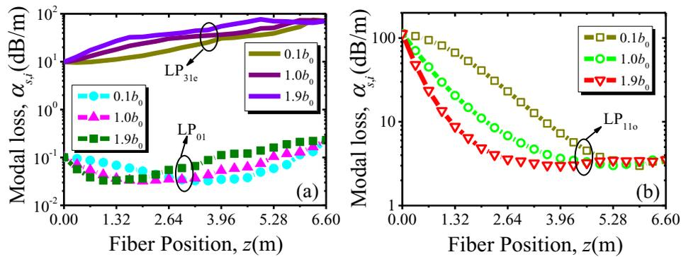
Figure 5. Comparison of modal loss of T-SCF with a bending radius of 32 cm: (a) mode losses of LP<sub>01</sub> and LP<sub>31e</sub>; (b) mode loss of LP<sub>11o</sub>.
