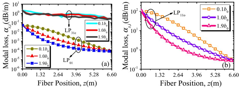
Figure 4. Comparison of modal loss of straight T-SCF from the small end to the large end: (a) mode losses of LP<sub>01</sub> and LP<sub>31e</sub>; (b) mode loss of LP<sub>11o</sub>.
