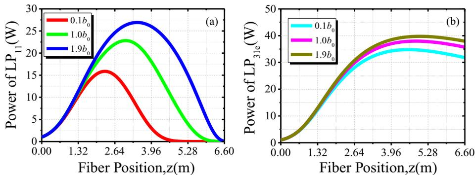
**Figure 14.** Modal power evolution of (a) LP<sub>11</sub> mode and (b) LP<sub>31e</sub> mode for concave, linear, and convex T-SCF under the large-to-small amplification scheme.
