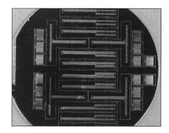
This silicon wafer contains three of five components fabricated for use in one integrated microchip for DNA analysis. Individual components in the microchip include entry ports, transport channels, a thermally controlled reactor where mixing and enzyme digestion or polymerase chain reaction amplification occurs, an electrophoresis channel, and a detector.
