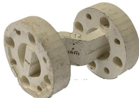
Fig. 12. Manufactured through-type structure for estimating attenuation of test fixture.
