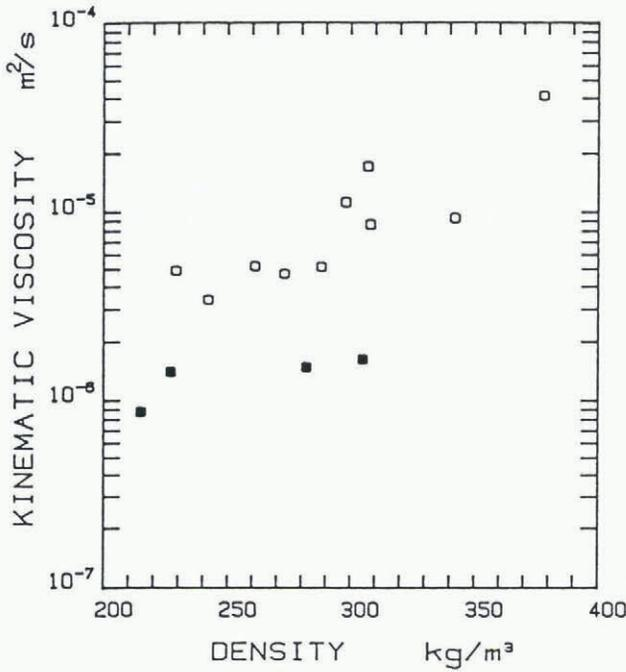
Fig. 8. Kinematic viscosity measurements for fluidized snow.
