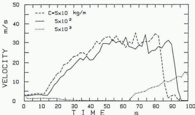
Fig. 10. Variations in calculated velocities of snow along the avalanche chute. Values of parameters selected except  $C$  are the same as in Figure 9.
