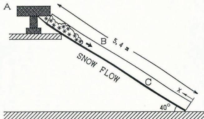
Fig. 1. Schematic diagram showing the experimental arrangements. A, fluidized-snow feeder; B, chute; C, sandpaper.
