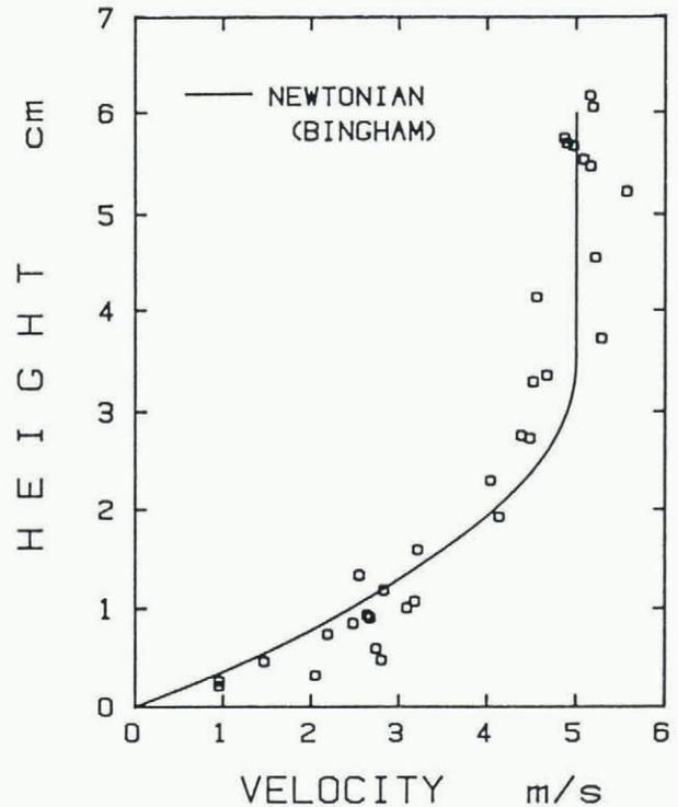
Fig. 4. Measured and calculated velocity profiles for flowing snow on the surface of packed snow.
