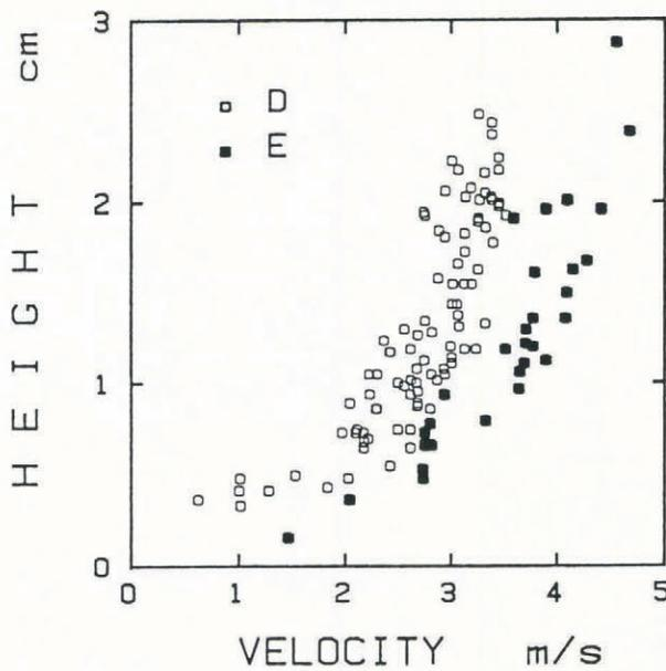
Fig. 6. Velocity profiles for snow flow in the regions D and E in Figure 5.
