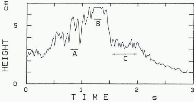
Fig. 2. Variation in snow-flow depth with time; results obtained from low-temperature laboratory experiments.
