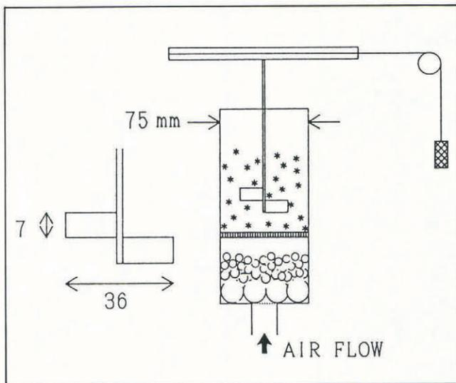
Fig. 7. Schematic diagram of the experimental apparatus for generating fluidized snow and for measuring its viscosity.
