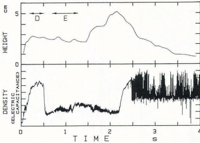
Fig. 5. Correlation between snow-flow depth and bulk density of snow at a depth of 0-20 mm.
