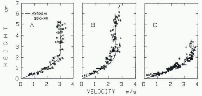
Fig. 3. Measured and calculated velocity profiles for flowing snow in the regions A, B, and C in Figure 2.
