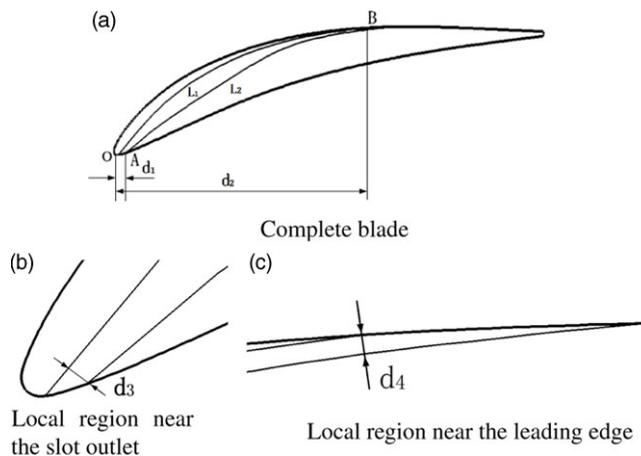
**Figure 3.** Slot structure.
