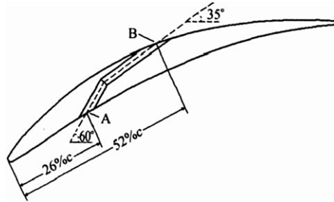
**Figure 1.** Convergent turning slot of two-segments [12].
