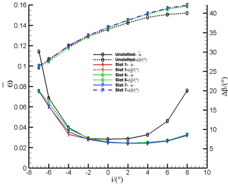
Figure 16. Performance of cascades with different slot shapes.
