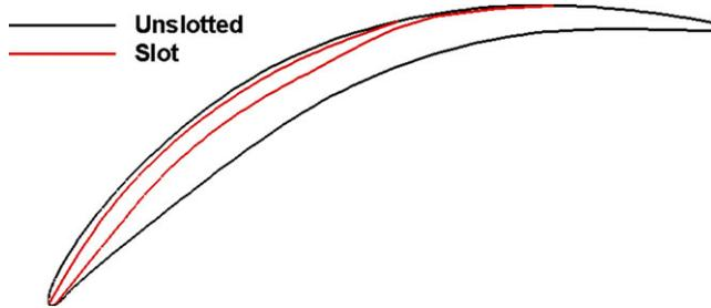
**Figure 24.** The more highly loaded cascade.
