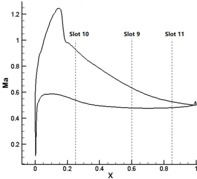
**Figure 21.** Distribution isentropic Mach numbers on the surfaces of an unslotted blade and the outlet slot positions.
