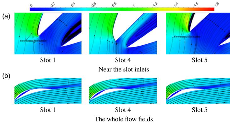
**Figure 12.** Mach number contours at an attack angle of 6 degrees.
