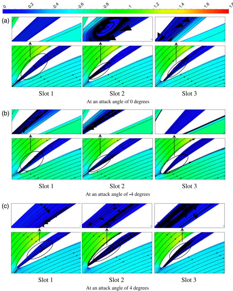
**Figure 9.** Mach number contours near the leading edges.
