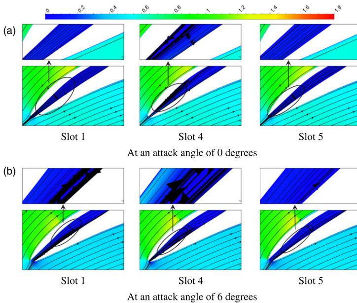
Figure 11. Mach number contours near the leading edges.
