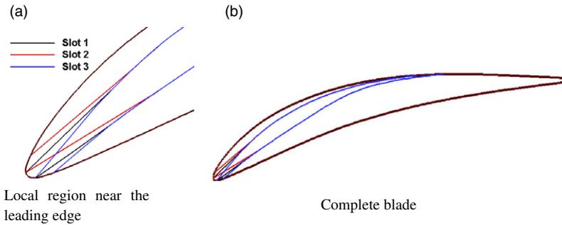
**Figure 7.** Inlet locations of the slots.
