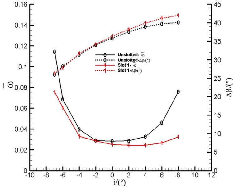
Figure 5. Performance of the unslotted and slotted cascades.
