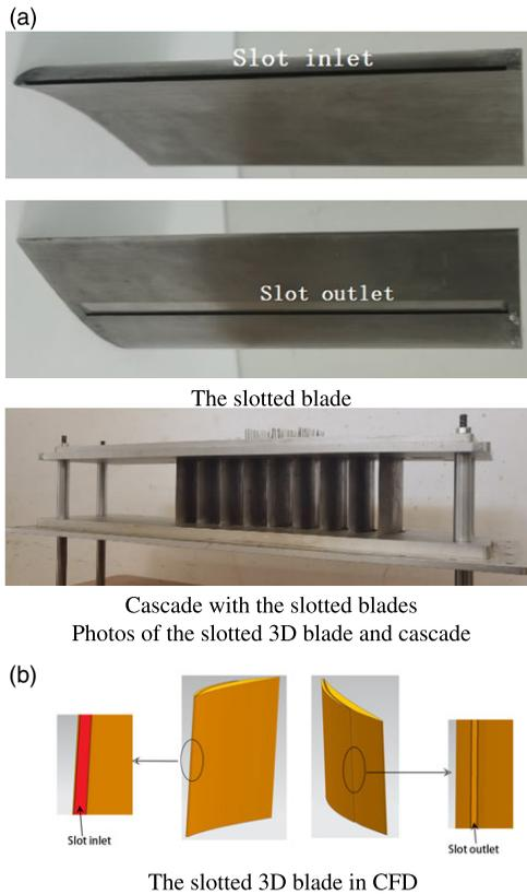
Figure 29. The 3D slotted blade.
