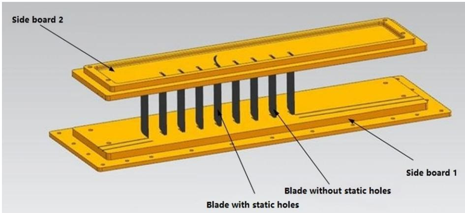
Figure 28. Three-dimensional view of the cascade.
