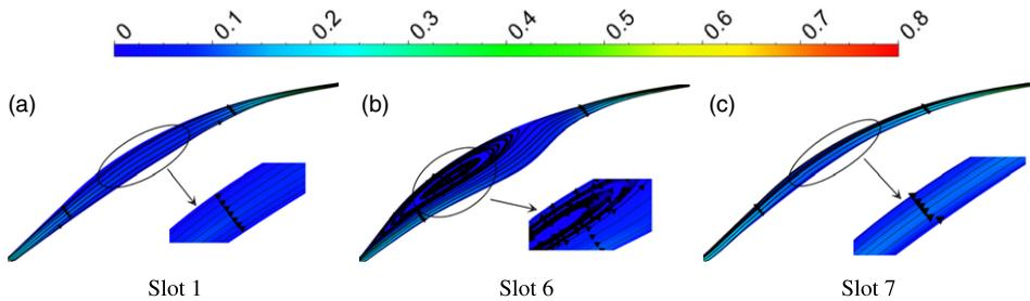
Figure 17. Mach number contours and streamlines.
