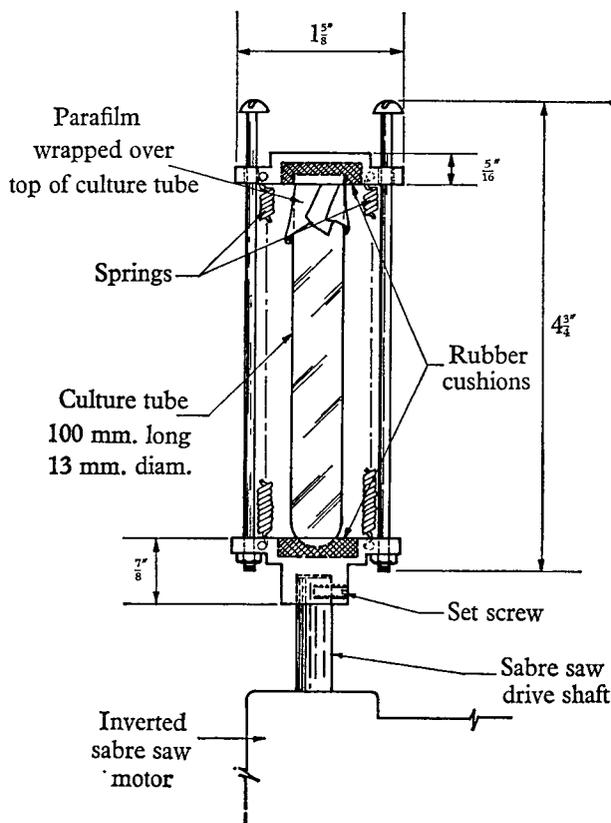
Fig. 1. Diagram of blender showing essential parts and typical dimensions.
