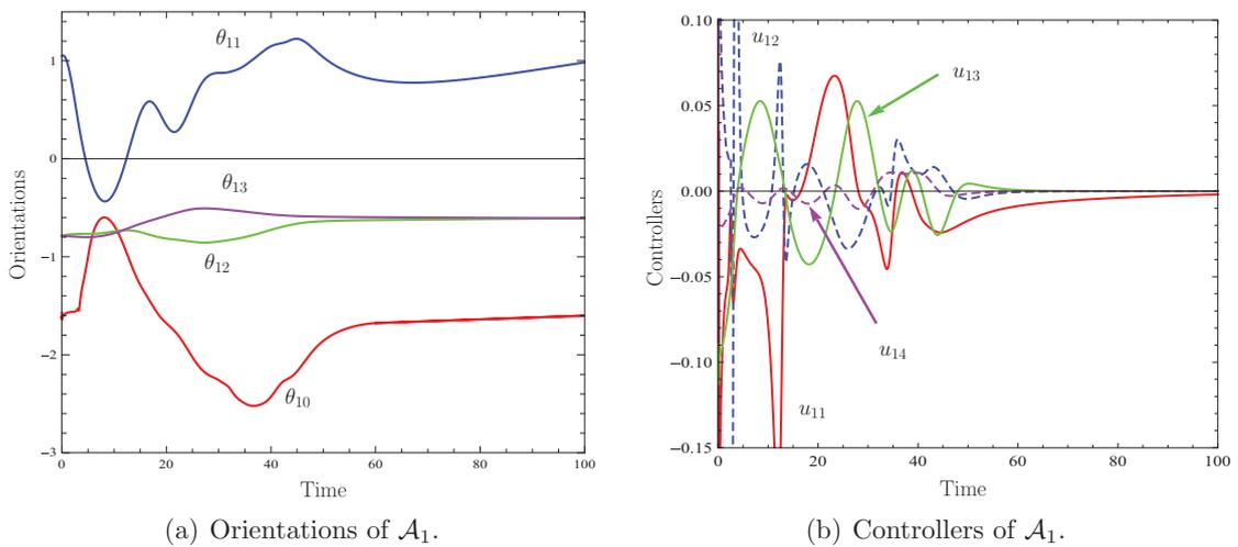
Fig. 8. Scenario 1. (a) portrays the evolution of the orientations of the various bodies of  $\mathcal{A}_1$ , while (b) depicts the evolution of its decentralized acceleration controls. (a) Orientations of  $\mathcal{A}_1$ . (b) Controllers of  $\mathcal{A}_1$ .
