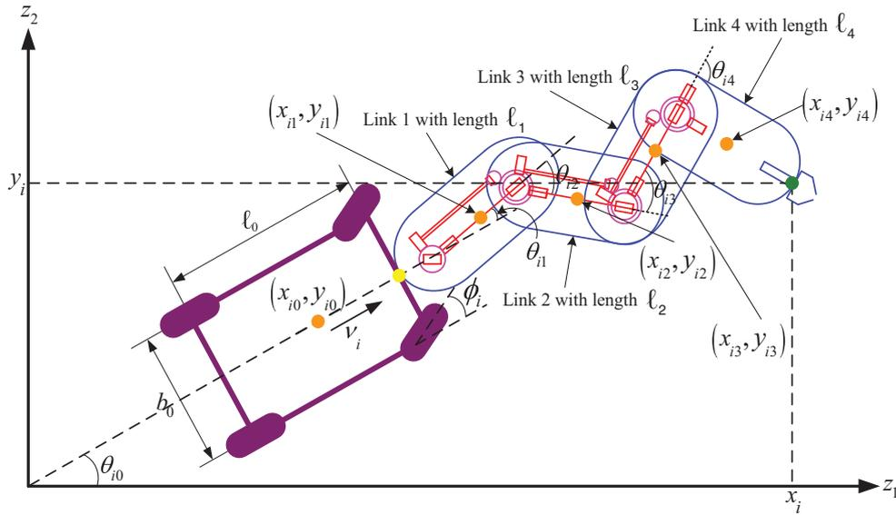
Fig. 1. Illustration of the  $i$ th 4DNM in the inertial frame  $\mathcal{F}$ . The schematics of the 4-link nonholonomic manipulator is adopted from.<sup>29</sup>
