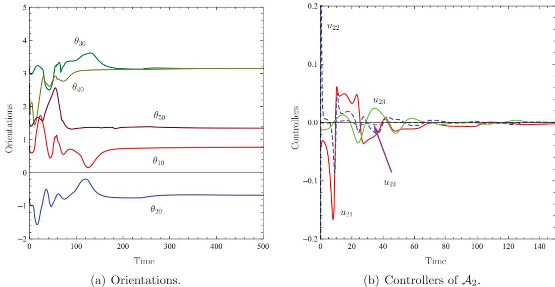
Fig. 10. Scenario 2. (a) shows the evolution of the orientations of the wheeled platforms of the 3DNMs while (b) depicts the progression of the acceleration controllers of  $\mathcal{A}_2$ . (a) Orientations. (b) Controllers of  $\mathcal{A}_2$ .
