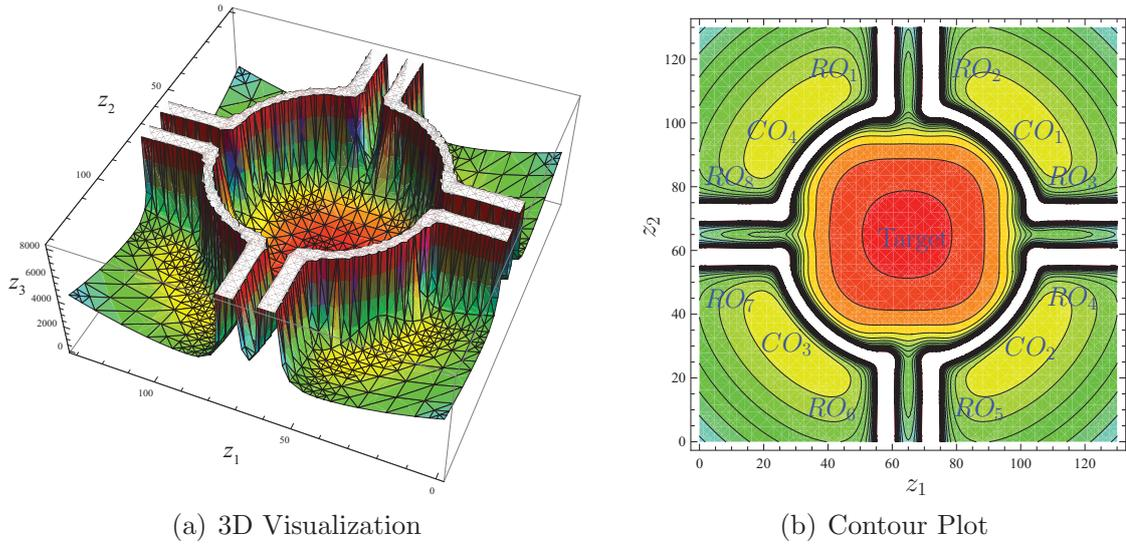
Fig. 6. The total potentials (corresponds to the  $z_3$ -axis) for target attraction and avoidance of multiple rod-shaped and curve-shaped obstacles by the wheeled platform of a 3DNM with the target fixed at  $(p_{11}, p_{12}) = (65, 65)$ . Also,  $v_1 = 2$ ,  $\omega_{10} = \omega_{11} = \omega_{12} = \pi/360$ ,  $\theta_{10} = 0$ ,  $\theta_{11} = \pi/3$ ,  $\theta_{12} = -\pi/3$ , and  $\theta_{13} = -\pi/4$ . (a) 3D visualization. (b) Contour plot.
