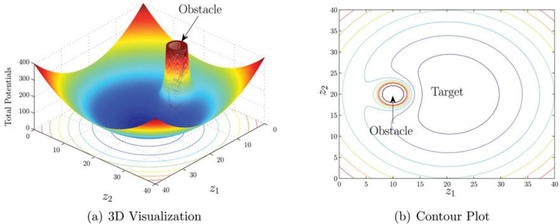
Fig. 3. The total potentials generated by Eq. (4). The target is located at  $(p_1, p_2) = (20, 20)$  with radius  $r_T = r_P = 1$  and the obstacle is fixed at  $(o_1, o_2) = (10, 20)$  with a radius of  $r_O = 2$ . The value of the tuning parameter is chosen as  $\alpha = 10$ . (a) 3D Visualization. (b) Contour plot.
