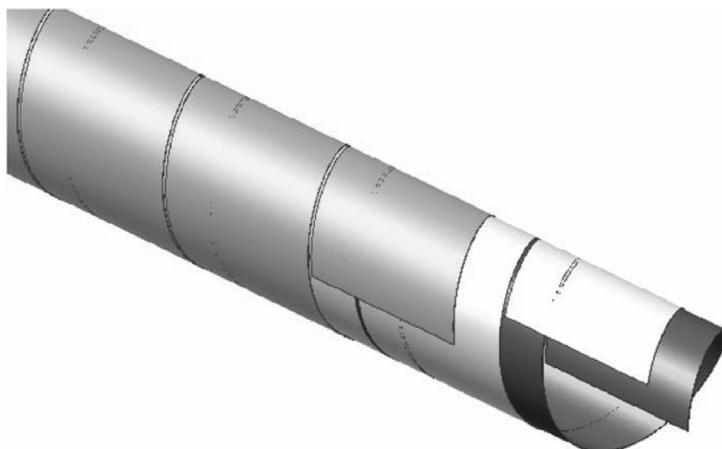
Figure 11.14 Two-layer structure of the straws for COMPASS (Bychkov *et al.*, 2006). By kind permission of Elsevier.
