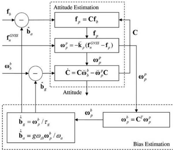
Figure 1. Bias Observer Block Diagram.
