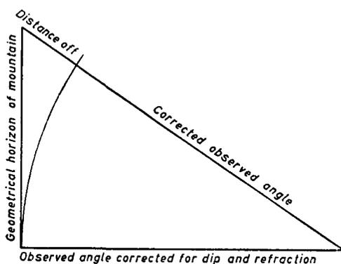
FIG. 1. Mnemonic showing relationship between height of mountain peak, angle observed and distance off.
