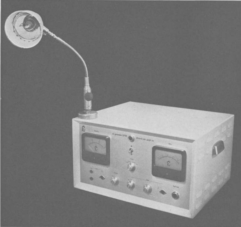
The Ahrend Van Gogh Laryngostroscope ( $\Delta$  F Generator) shows the vibration of the vocal chords slowed down to about one cycle per second. It is also possible to stop the movement by stroboscopic effect and then tune through all phases of one cycle.
