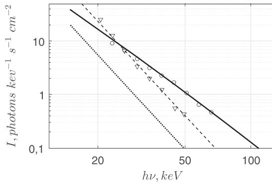
**Figure 2.** Observed and calculated hard X-ray spectra for the July 19, 2012 solar flare. The results of modelling the chromospheric source are represented by the straight solid line; the observations are indicated by the circles. The results of modelling the coronal source without and with allowance for the electron acceleration in the collapsing magnetic trap are represented by the dotted and dashed straight lines, respectively; the observations are indicated by the triangles.
