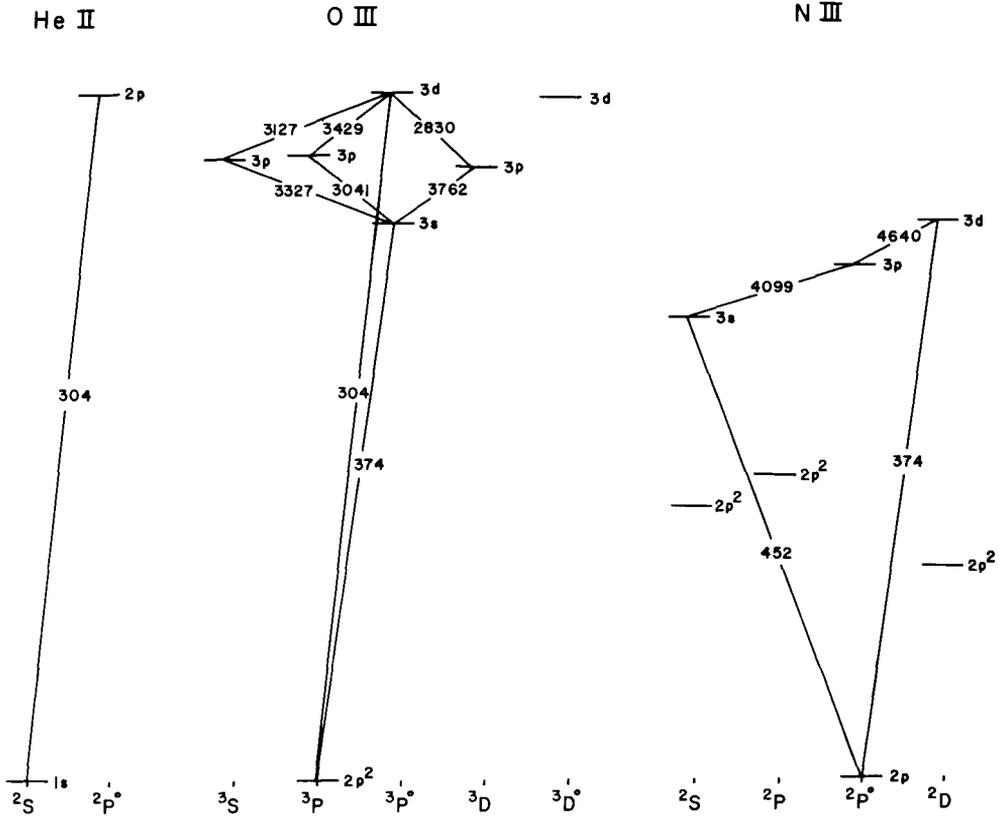
Figure 1 -- Partial energy level diagrams for He II, O III, and N III showing the transitions involved in the Bowen fluorescence mechanism.
