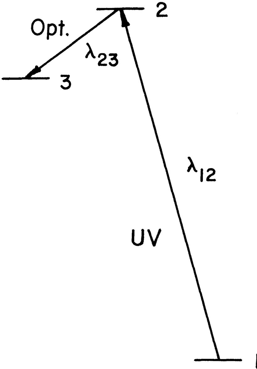
Figure 6 -- Schematic energy level diagram for transitions excited by resonance fluorescence of continuum radiation.
