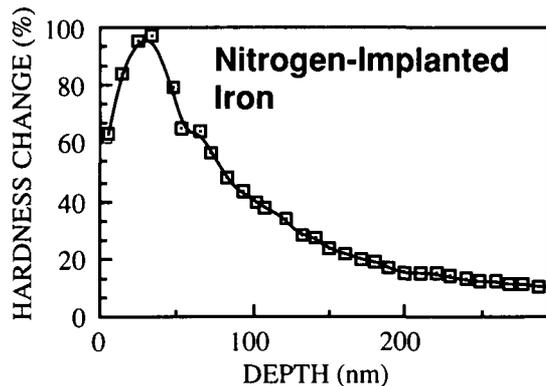
Hardness change produced by a 150 nm thick layer of implanted nitrogen on an iron sample.
