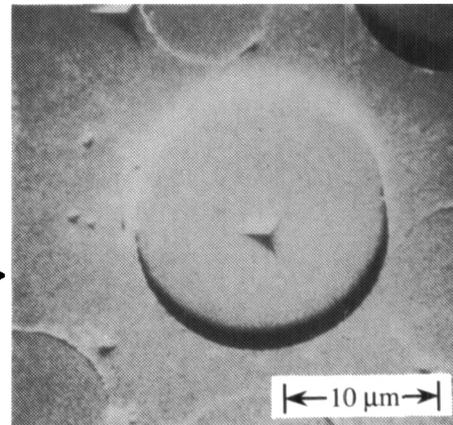
Fiber sliding is used to characterize ceramic-fiber composite interfaces.
