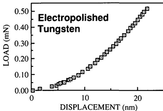
Repeated loadings/unloadings of an elastic contact shows the extreme displacement and load resolution achieved by the Nano Indenter.
