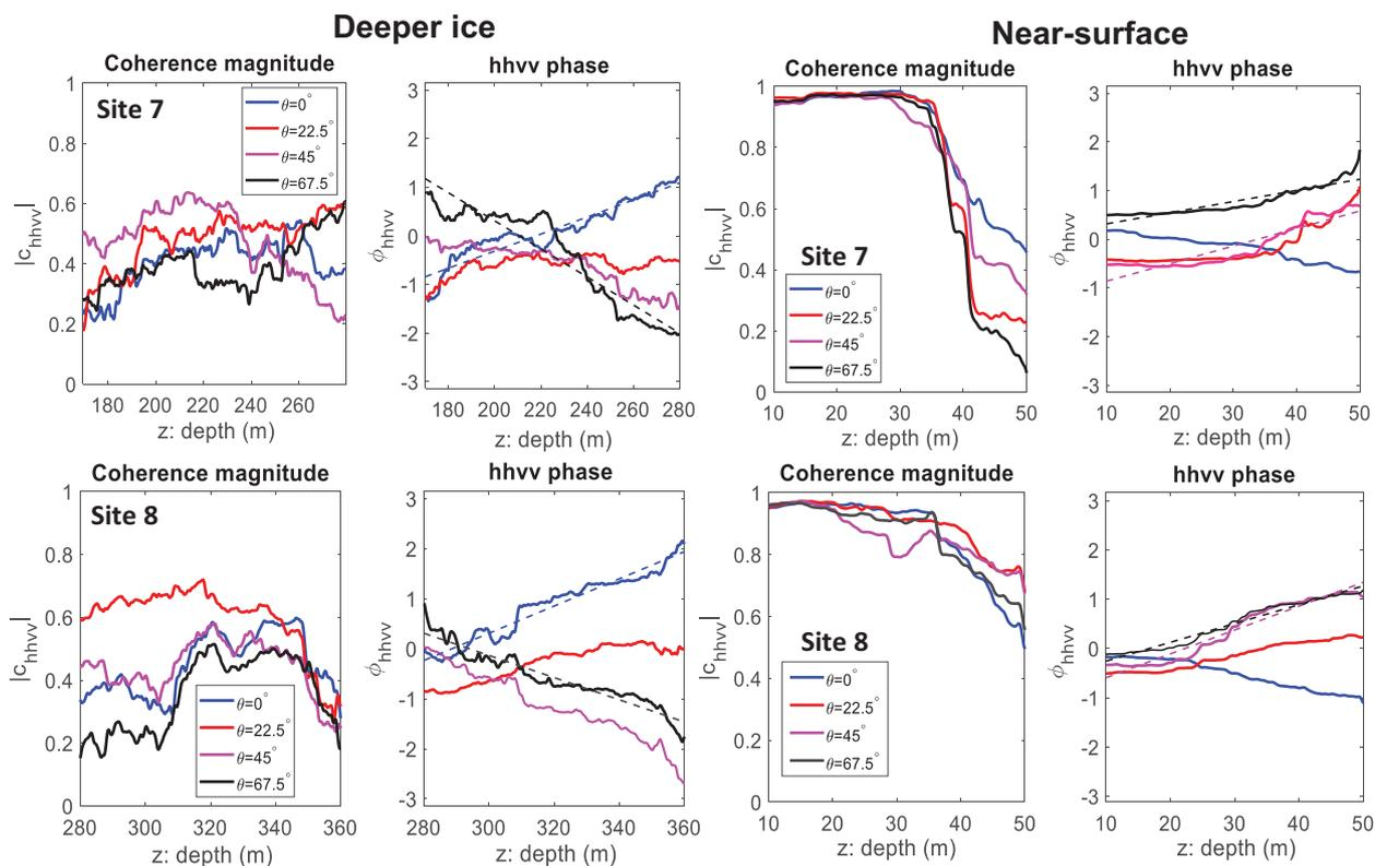
**Fig. 8.** Ice fabric estimates at sites 7 and 8 using the vertical phase gradient method. The regression lines (angles either side of the inferred principal axis) that are used to estimate the  $E_2 - E_1$  eigenvalue difference are indicated.
