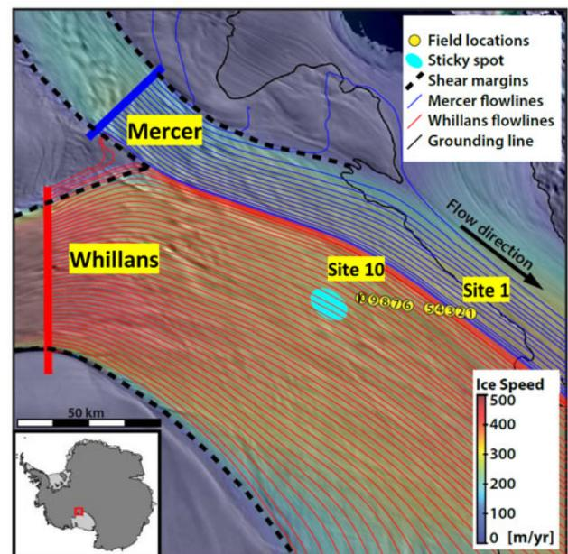
Fig. 1. Field setting of Whillans and Mercer ice streams on the Siple Coast, West Antarctica. The radar ground survey measurement sites are shown as numbered yellow dots. Streamlines from Whillans (red) and Mercer (blue) ice streams are derived from ice velocity (Rignot and others, 2011, 2017). Background image shows ice velocity over a mosaic of MODIS visible satellite imagery (Haran and others, 2005).
