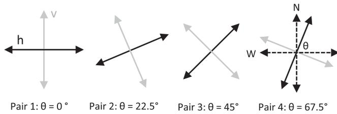
Fig. 3. Definition of  $h-v$  pairs in polarimetric coherence calculations.
