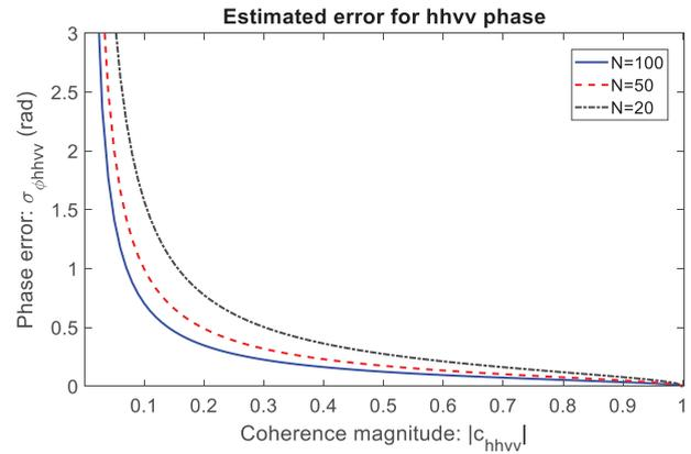
Fig. 4.  $hhvv$  phase error as a function of  $hhvv$  coherence magnitude and number of range bins,  $N$ .
