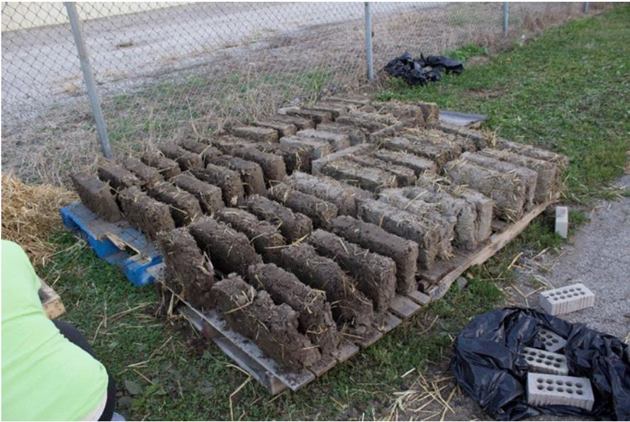
**Figure 2.** | Storage and drying of mudbricks at an off-campus facility.
