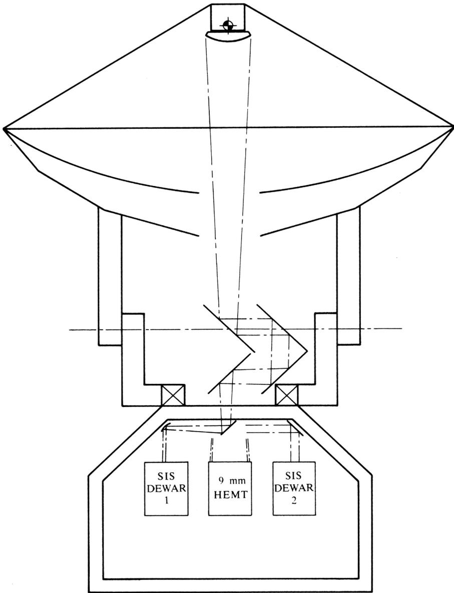
**Figure 3.5** Conceptual MMA antenna design. Plane mirrors guide the beam to one of three cryogenic dewars, two with SIS mixer receivers and one with a high electron mobility transistor (HEMT) amplifier receiver. Credit: NRAO/AUI/NSF, CC BY 3.0.
