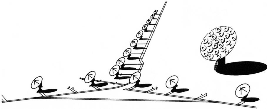
**Figure 3.2** First revision of the original MMA concept with the 6 m diameter antennas in a Y-configuration on tracks and the 3 m diameter antennas mounted on a steerable platform. Credit: NRAO/AUI/NSF, CC BY 3.0.
