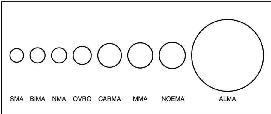
**Figure 3.3** The circles indicate the relative geometric collecting areas of the millimeter/submillimeter arrays that have been discussed, for comparison with the proposed MMA, as well as that of ALMA. The actual power of an array depends on additional factors: efficiency of the antenna optics, performance of the electronics, and quality of the atmosphere at the array site. Courtesy of Thomas van den Bout, reproduced by permission.
