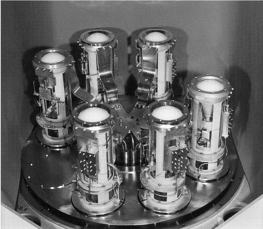
**Figure 3.6** The illustration on the cover of the first MMA Design and Development Plan was of a multi-beam receiver for the NRAO 12 Meter Telescope. The six receiver cartridges were cooled by a common refrigerator and held in a common cryogenic container, a scheme later used for ALMA. Credit: NRAO/AUI/NSF, CC BY 3.0.
