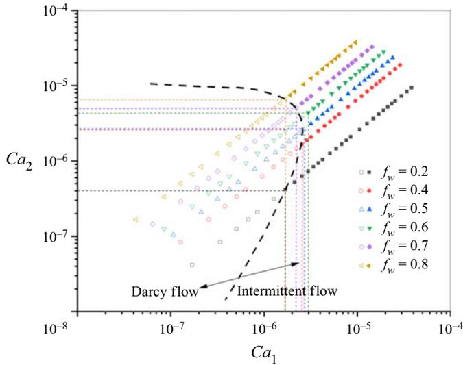
Figure 4. The phase diagram showing linear flow (empty symbols) and nonlinear flow (filled symbols) for sample A as a function of oil capillary number  $Ca_1^i$  and water capillary number  $Ca_2^i$ . The black dashed line is the predicted transition from Darcy to intermittent flow using (4.2) and (4.3).
