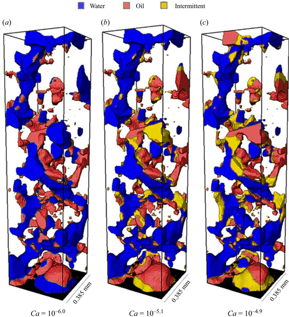
Figure 3. Three-dimensional views of the segmented phases on a  $100 \times 100 \times 400$  voxels sub-volume of the full image for  $f_w = 0.7$  and  $Ca = 10^{-6.0}$ ,  $10^{-5.1}$  and  $10^{-4.9}$ . Water is blue, oil is red and intermittent regions are shown in yellow.
