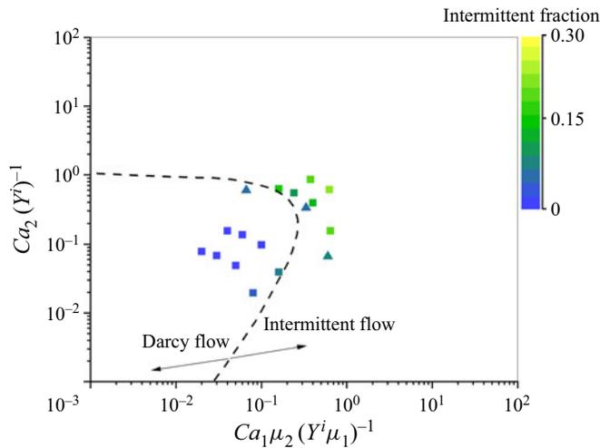
Figure 5. The replotted phase diagram showing the fraction of the pore space that has intermittent occupancy; the squares are for sample B, and the triangles are data from the literature (Zou *et al.* 2018). The dashed line is the predicted transition from Darcy to intermittent flow using (4.2) and (4.3).
