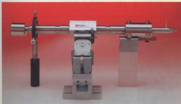
Simultaneously monochromatize and either focus or collimate an x-ray beam
