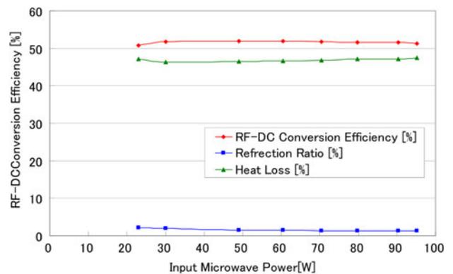
Fig. 12. RF-DC conversion efficiency of high-power rectenna in the case of 64-parallel connections and a load of 10 Ω.
