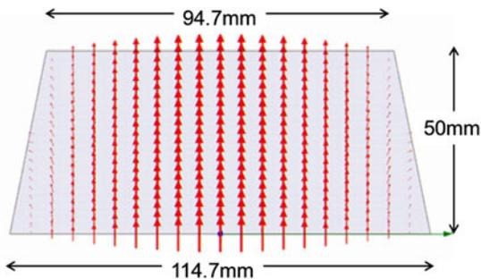
Fig. 4. Simulation result of the TE<sub>1,0</sub> mode traversing a deck plate waveguide.
