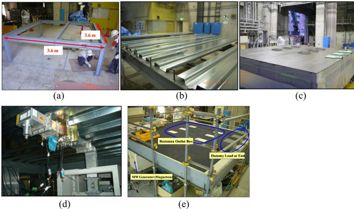
Fig. 18. Final test setup: (a) frame, (b) deck plate waveguide, (c) concrete at floor, (d) power distributor, (e) final setup.
