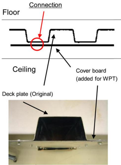
Fig. 3. Illustration and photograph of deck plate waveguide.
