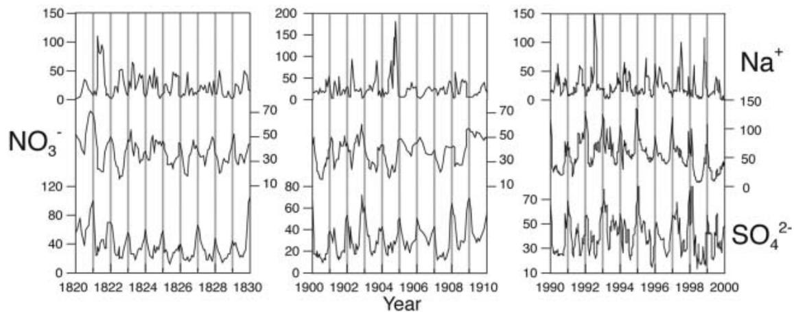
**Fig. 3.** Annual chemistry layers ( $\mu\text{g L}^{-1}$ ) from the 00-1 ice core used for dating. Detailed 10 year sections (1820–30, 1900–10, 1990–2000) display winter–spring ( $\text{Na}^+$ ) and summer ( $\text{NO}_3^-$ ,  $\text{SO}_4^{2-}$ ) maxima. Clear seasonal signals are present in all records.
