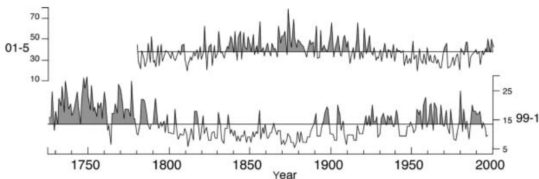
**Fig. 5.** Accumulation-rate records in  $\text{cm a}^{-1}$  w.e. for the full record for sites 01-5 and 99-1. The line through the record denotes the mean accumulation, and the shaded portions of the record are above mean accumulation. The trends may be due to topographical effects.
