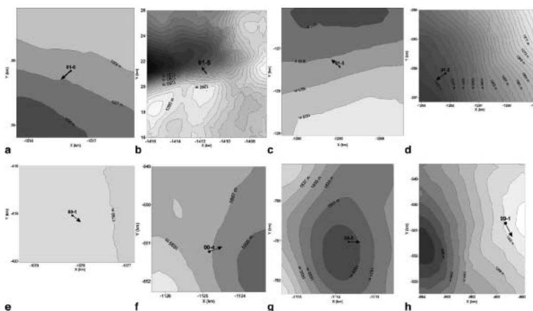
**Fig. 6.** Polar stereographic projections of the surface topography at sites (a) 01-6, (b) 01-5, (c) 01-3, (d) 01-2, (e) 00-1, (f) 00-4, (g) 00-5, (h) 99-1. Contour labels are in m at 2 m intervals. Arrows indicate ice flow vectors. Note: the area covered by the projections differs between sites.
