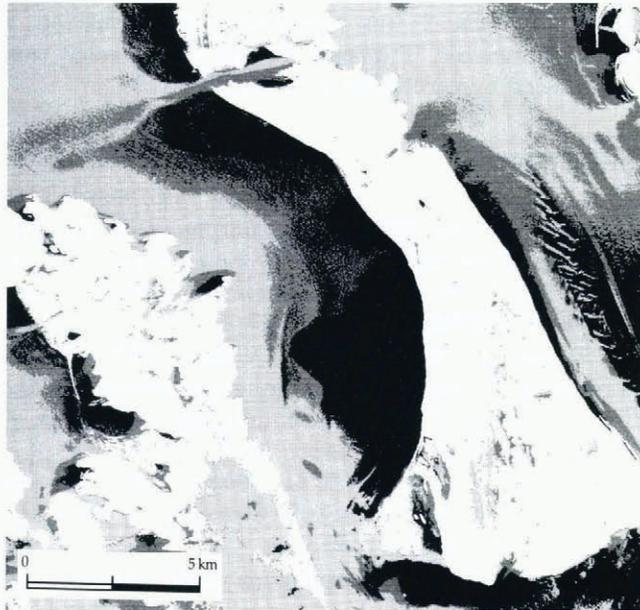
Fig. 8. Classification of SPOT scene 153-690 (8 February 1987) according to the decision tree classifier of Figure 6. Rock outcrops and morainic debris are displayed in white, bare glacier ice in black, ice covered with a layer of snowdrift (snow/ice) in grey and snow in light grey. See Figure 4 for situation.
