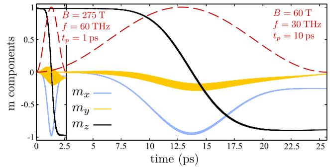
**Figure 4.** Micromagnetic simulation results of the temporal evolution of the magnetization components ( $m_x$  blue,  $m_y$  yellow,  $m_z$  black) of CoFeB excited by an RCP B-field. The normalized B-field envelope is shown in dashed red. While a B-field of  $B_0 = 60$  T,  $f = 30$  THz and  $t_p = 10$  ps shows switching at the ps timescale, a B-field of  $B_0 = 275$  T,  $f = 60$  THz and  $t_p = 1$  ps achieves it at the femtosecond timescale.
