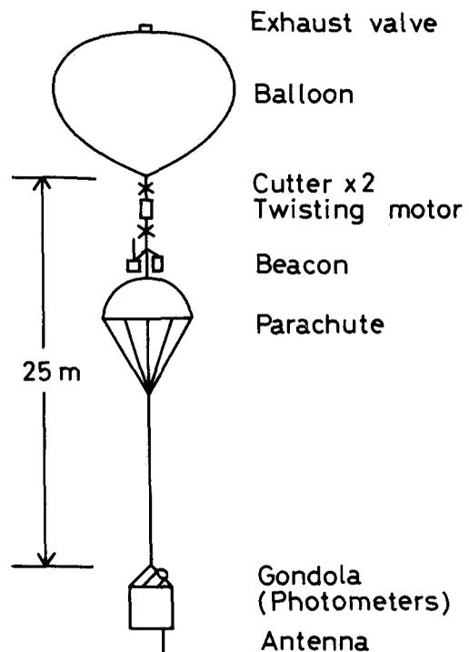
Figure 2. Construction of the Balloon.
