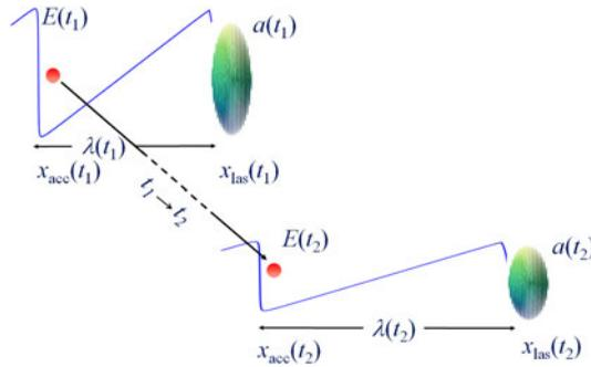
FIGURE 13. The wavelength and electric field amplitude changes being different at different times  $t_1$  and  $t_2$  due to the change of plasma density leading to a change in the laser pulse parameters. For a matched plasma density profile, the accelerated electrons remain in the acceleration phase of the wake field.
