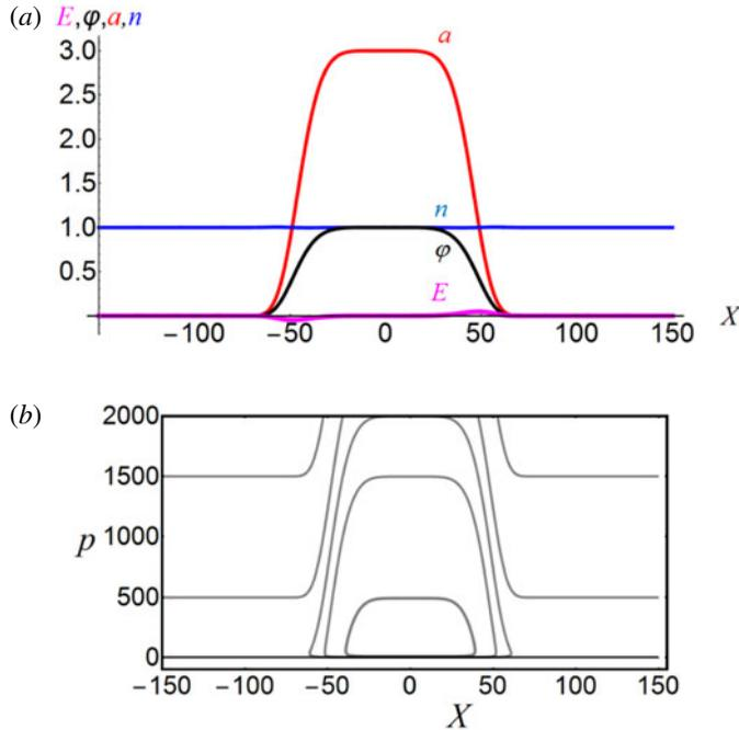
FIGURE 10. (a) Electrostatic potential, electric field, electron density and the laser pulse (dashed line) versus the coordinate  $X$ . (b) The electron phase plane ( $X, p$ ). The laser pulse corresponding to the trial potential  $\varphi_a$  given by (3.32) having index  $2q=6$ , length  $L=50$  and amplitude  $F=1$  propagating in a plasma characterized by  $\beta_w=0.9995$  ( $\gamma_w=31.6$ ).
