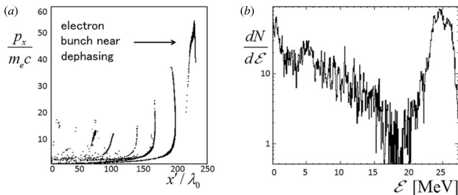
FIGURE 22. (a) Electron phase space  $(x', p_x)$  and (b) energy spectrum at  $t = 2000$ ; the  $x'$  axis is normalized by the laser wavelength  $\lambda_0$  which is expressed in terms of the simulation box coordinates,  $x' = x - ct$ , and the momentum  $p_x$  is normalized by  $m_e c$ .
