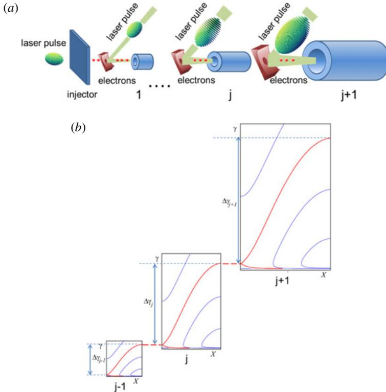
FIGURE 18. Multi-uneven stage accelerator comprising the injector and unequal stages. (a) Schematic of the multi-unequal stage LWFA accelerator. (b) Phase plots ( $X, \gamma$ ) corresponding to the  $j - 1$ th,  $j$ th and  $j + 1$ th stages of the accelerator.
