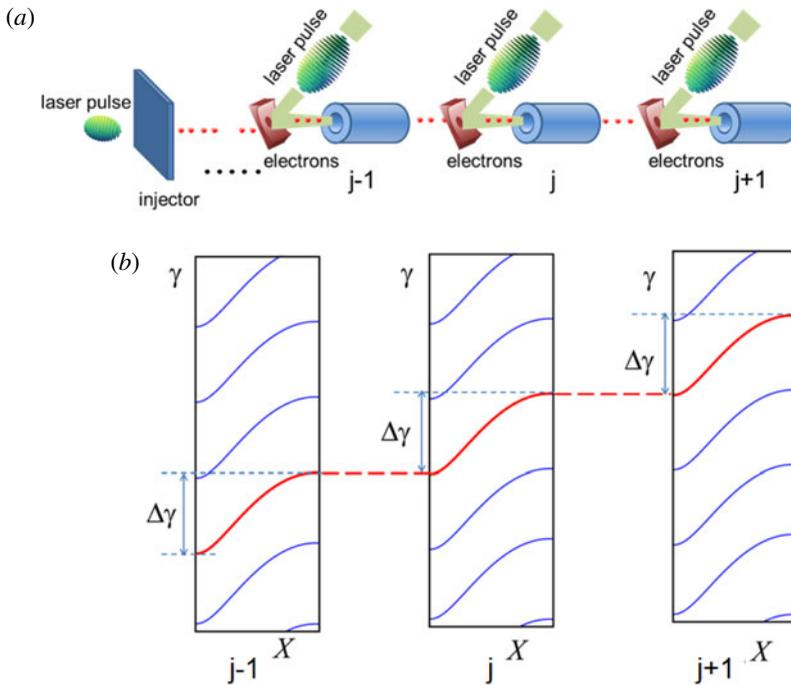
FIGURE 17. Multi-even stage accelerator comprising the injector and equal stages. (a) Schematic of the multi-equal stage LWFA accelerator. (b) Phase plots ( $X, \gamma$ ) corresponding to the  $j - 1$ th,  $j$ th, and  $j + 1$ th stages of the accelerator.
