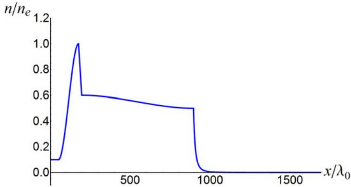
FIGURE 19. Plasma density profile with a sharp density gradient of width  $20\lambda_0$  at  $x = 175\lambda_0$  (injector) and a sharp density drop off at  $x = 895\lambda_0$  (end of phase rotation and acceleration) along the laser propagation direction with the laser entering from the left. The density is normalized by the peak plasma density  $n_e$  and the propagation distance is normalized by the laser wavelength  $\lambda_0$ .
