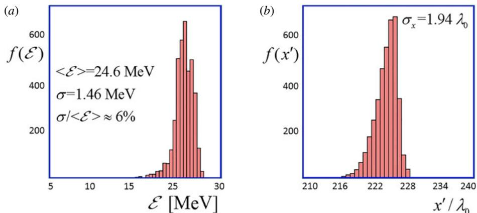
FIGURE 23. (a) Electron spectrum and (b) electron bunch profile of the first bunch in figure 21; the  $x'$  axis is normalized by the laser wavelength  $\lambda_0$ , which is expressed in terms of the simulation box coordinates,  $x' = x - ct$ .
