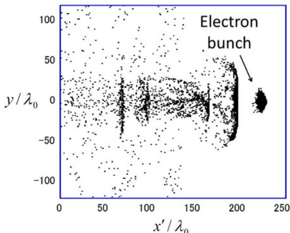
FIGURE 21. Density distribution of electrons in the plane  $(x, y)$  after the laser has exited the plasma (practically in vacuum) at  $t=2000$  which is normalized by  $2\pi/\omega_0$ . An electron bunch (indicated by the arrow) can be seen on the right side of the simulation box where the density is normalized by the peak plasma density  $n_e$  and the  $x'$  and  $y$  axes are normalized by the laser wavelength  $\lambda_0$ . Here  $x' = x - ct$  is the coordinate used in simulation.
