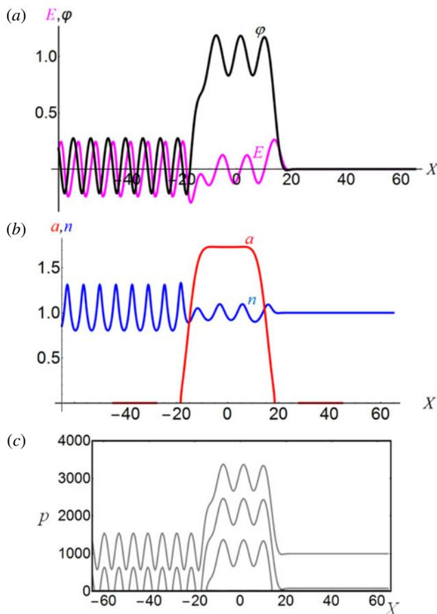
FIGURE 11. The same is in figure 10 for the laser pulse corresponding to the trial potential  $\varphi_a$  given by (3.32) having index  $2q = 6$ , length  $L = 15$  and amplitude  $F = 1$  propagating in a plasma characterized by  $\beta_w = 0.9995$  ( $\gamma_w = 31.6$ ).
