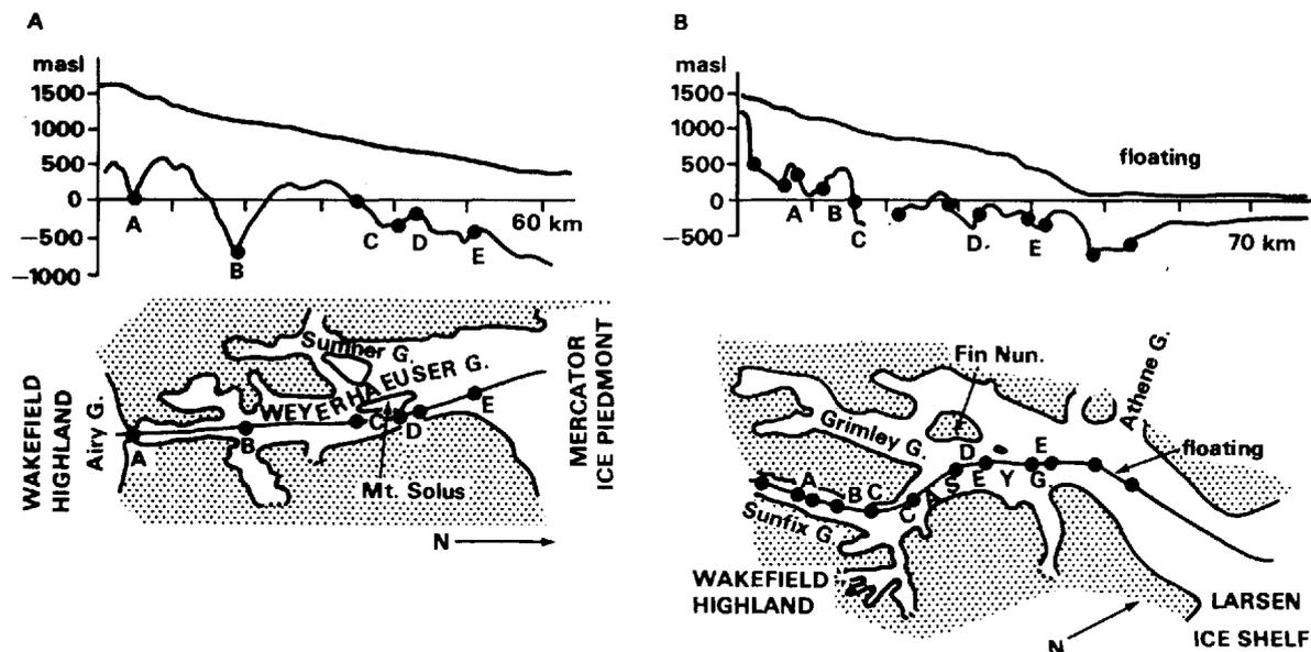
Fig.2. Long profiles of Weyerhaeuser (A) and Sunfix and Casey glaciers (B). Heavy dots relate features on the profiles to their position along the flight tracks. Vertical exaggeration is x 10.
