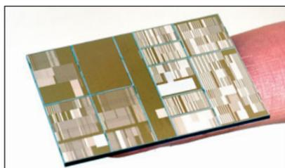
One of the nanotechnology-inspired grand challenges suggested by the White House is to create computer chips that are 100 times faster yet consume less power. This picture shows a computer chip with 7-nm transistors that IBM made by using silicon-germanium instead of silicon. The technology could enable up to 20 billion transistors on a fingernail-sized chip. Credit: Darryl Bautista/Feature Photo Service/IBM.
