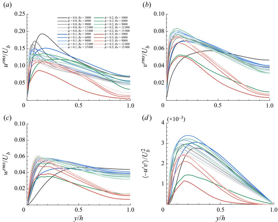
Figure 3. Wall-normal profiles of (a) streamwise, (b) wall-normal and (c) spanwise fluid velocity r.m.s. (d) Wall-normal profiles of the Reynolds stress. All panels are in outer scale.
