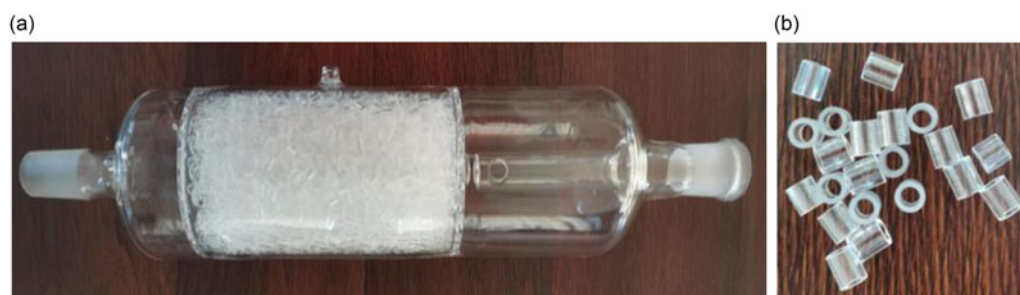
Figure 3. (a) Raschig tube and (b) glass Raschig rings.
