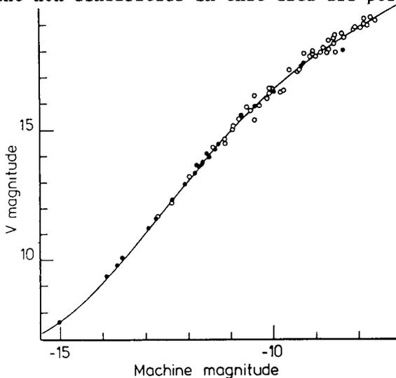
Figure 2 - A Schmidt plate calibration curve using standards from photoelectric and CCD observations (open points and all with  $V < 12$ ) and sub-beam prism plates (solid points). The curvature is evident.
