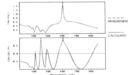
A cross comparison between Spectroscopic Ellipsometry and X-TEM gives very good agreement and show a better resolution of the multilayer structure.
