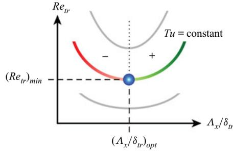
FIGURE 12. Sketch shows the scale-matching model, based on the hypothesis that, for each  $Tu$ , there exists an optimal  $\Lambda_x/\delta_{tr}$  that promotes transition to a lowest possible  $Re_{tr}$ .
