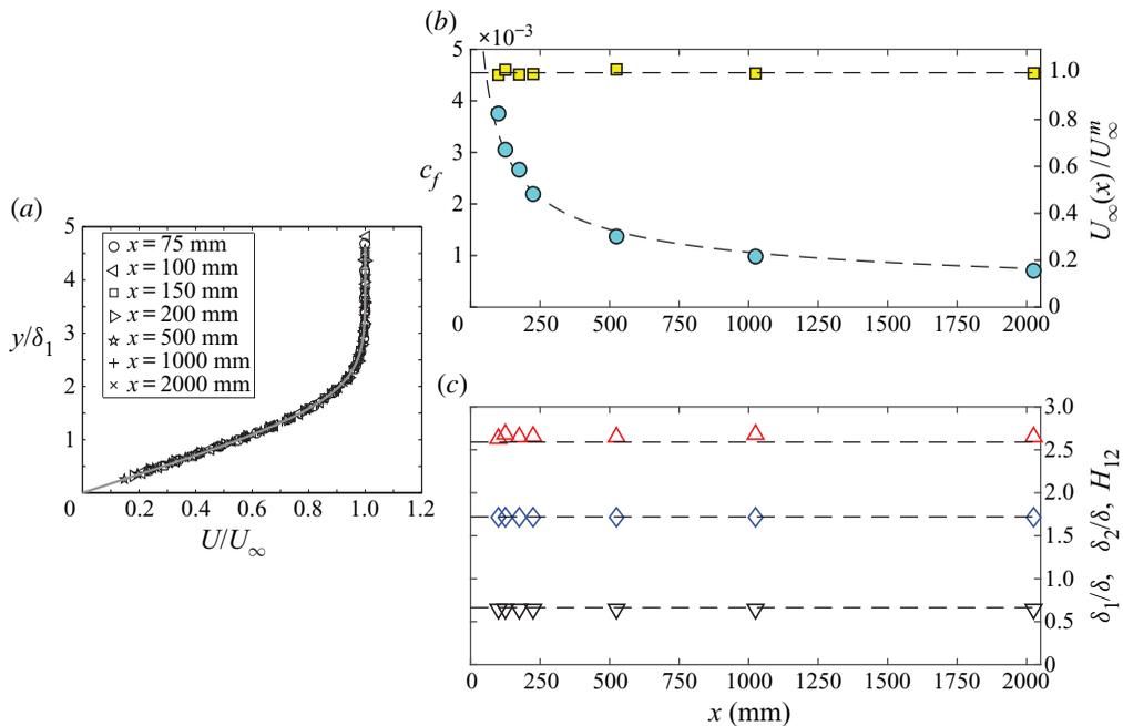
FIGURE 2. Base flow over the flat plate boundary layer. (a) Wall-normal mean velocity profiles at different  $x$ -locations. (b) Streamwise skin-friction ( $\circ$ ) and free-stream velocity ( $\square$ ) evolution. (c) Integral boundary-layer parameters: shape factor  $H_{12}$  ( $\Delta$ ), displacement thickness  $\delta_1$  ( $\diamond$ ) and momentum thickness  $\delta_2$  ( $\nabla$ ). Solid and dashed lines correspond to the Blasius boundary-layer solution.
