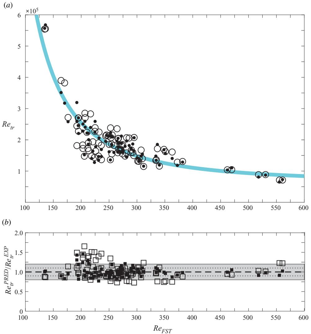
FIGURE 15. (a) Qualitative comparison between the measured transitional Reynolds number (open circles) and the corresponding predicted values (black circles) versus  $Re_{FST}$ . The solid line corresponds to (3.6). (b) Predicted values with respect to the measured values, from (4.7) and (3.6) with black square symbols and open squares, respectively.
