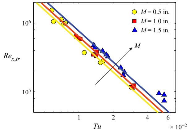
FIGURE 1. Transitional Reynolds number versus turbulence intensity for three different turbulence generating grids with increasing mesh width ( $M$ ), from  $M = 0.5$  to  $1.5$  in. Experimental data by Hislop (1940).
