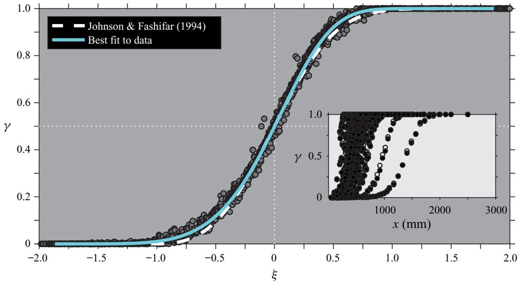
FIGURE 5. All 84 intermittency distributions from hot-wires 1 and 2 are shown in the scaled streamwise coordinate  $\xi$ . Dashed and solid lines correspond to the Johnson & Fashifar (1994) distribution and the best sigmoid curve fit to the data, respectively. The inset shows all intermittency distributions unscaled, filled and open symbols correspond to hot-wire probes 1 and 2, respectively.
