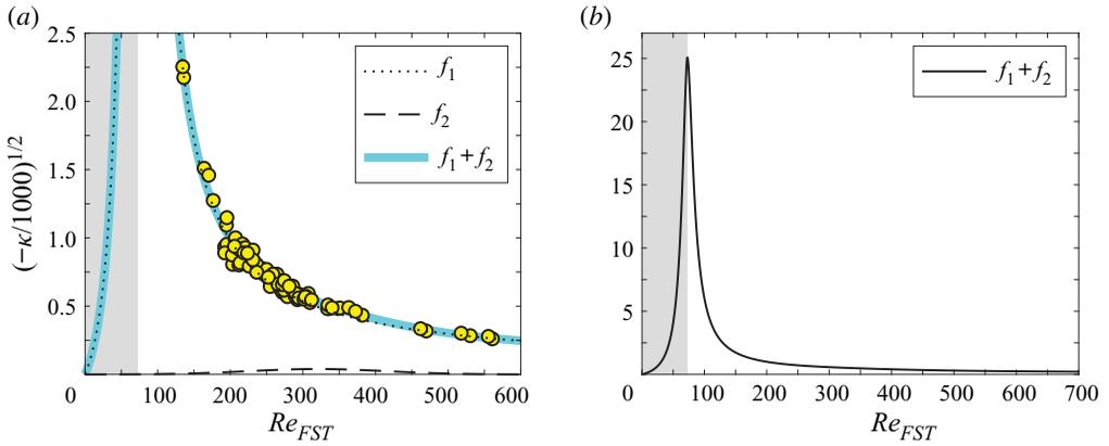
FIGURE 13. Weighting function  $\kappa$  versus  $Re_{FST}$ . (a) Close up of the  $\kappa$ -function according to (4.10), symbols correspond to experimental data. (b) Full  $\kappa$ -function produced by (4.10) for the range  $Re_{FST} = 0-700$ . Grey regions correspond to  $Re_{FST} \leq 73$ , which by combining (3.5) and (3.6) leads to  $Tu \leq 1\%$ .
