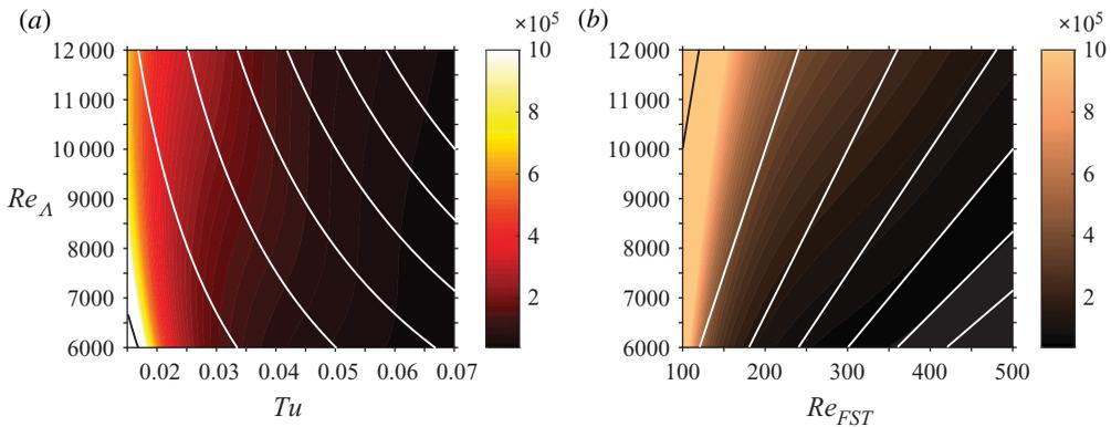
FIGURE 17. Contour plots of predicted transitional Reynolds numbers by (4.7). (a)  $Re_\Lambda$ – $Tu$  plane, with contour lines corresponding to  $Re_{FST} = 100:100:700$ , from left to right. (b)  $Re_\Lambda$ – $Re_{FST}$  plane, with contour lines corresponding to  $Tu = 0.01:0.01:0.07$ , from left to right.
