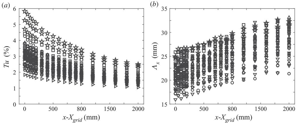
FIGURE 3. Free-stream turbulence intensity decay (a), and longitudinal integral length scale (b) in the streamwise direction for cases C1–C42 in table 2. Here  $X_{grid}$  corresponds to the distance between the grid and the leading edge for each case, with the origin at the grid location. For symbol definitions, see table 1. The different streamwise evolution curves have been generated by changing  $X_{grid}$  and the injection rate for the active grids.
