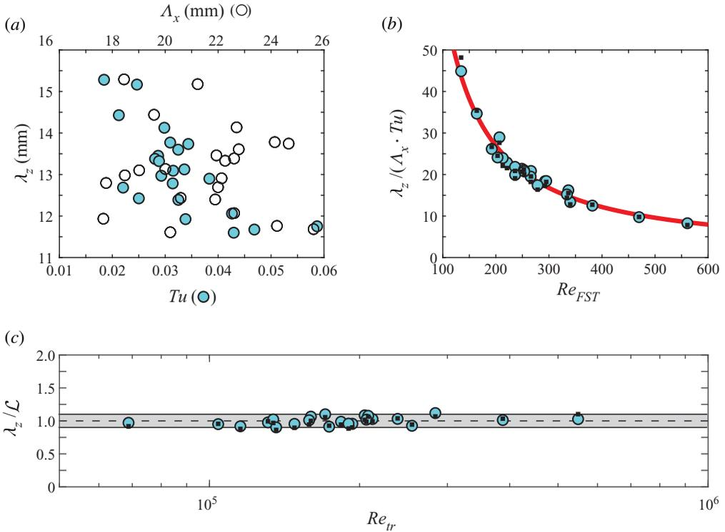
FIGURE 10. Averaged spanwise wavelength of the streamwise streaks. Panels (a) and (b) show unscaled and scaled wavelengths versus  $Tu$  and  $\Lambda_x$  and  $Re_{FST}$ , respectively. Panel (c) indicates the accuracy in estimating  $\lambda_z$  using (3.7) for different transitional Reynolds numbers. The solid lines correspond to deviations of  $\pm 10\%$  from the dashed line. Circular and square symbols correspond to streamwise locations of  $\gamma = 0.5$  and  $0.1$ , respectively.
