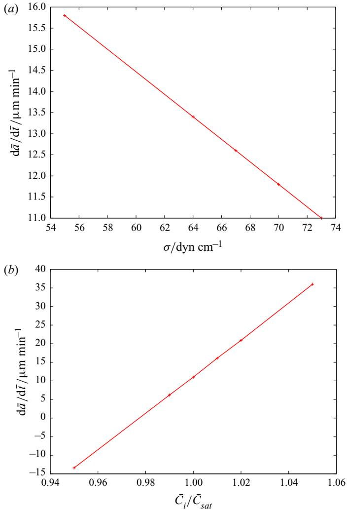
Figure 4. The time-averaged rate of growth of the mean value of the equilibrium bubble radius,  $d\bar{a}/d\bar{t}$ , using a numerical solution of the simplified mathematical model (3.27)–(3.29a–c) with  $\bar{R}_{eqi} = 40 \mu\text{m}$  for (a) a range of values for the surface tension and (b) a range of values of the initial uniform concentration of the gas in the liquid.
