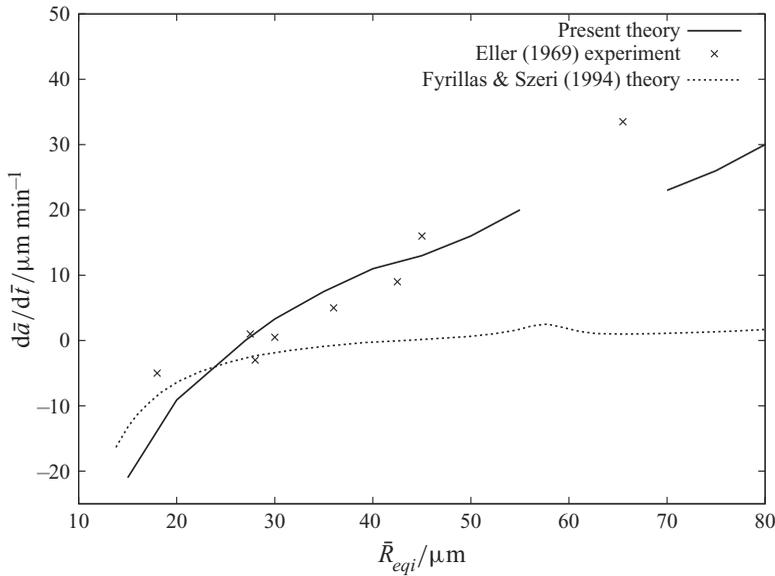
Figure 3. Comparison of the time-averaged rate of growth of the mean value of the equilibrium bubble radius,  $d\bar{a}/d\bar{t}$ , using a numerical solution of the simplified mathematical model (3.27)–(3.29a–c), the experimental results of Eller (1969) and the theoretical results of Fyrillas & Szeri (1994). In the experiment, a bubble in air-saturated water is subject to a sound field of 26.6 kHz.
