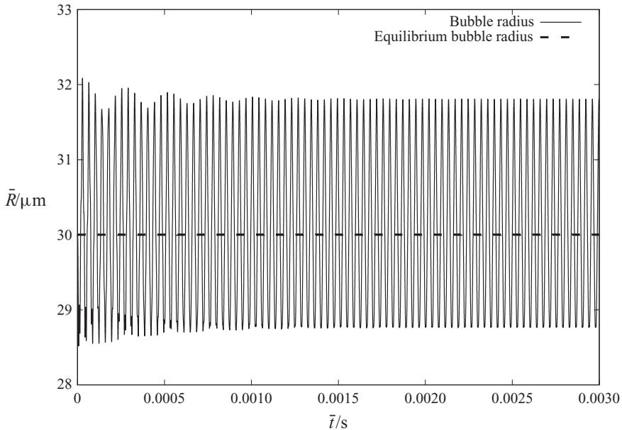
Figure 2. The bubble radius,  $\bar{R}$ , and the equilibrium bubble radius,  $\bar{R}_{eq}$ , using a numerical solution of the simplified mathematical model (3.27)–(3.29a–c) and an initial equilibrium bubble radius of  $\bar{R}_{eqi} = 30 \mu\text{m}$  corresponding to figure 1(a).
