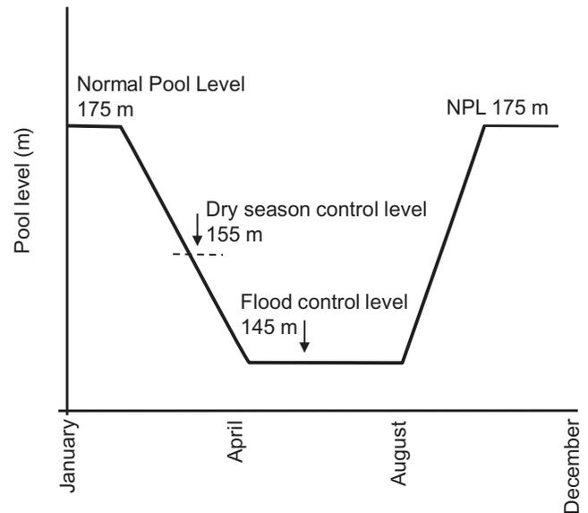
Figure 4.49. Seasonal pool operation at Three Gorges Dam, Yangtze River, China. Drawdown procedure results in pool lowering by some 30 m during the flood season relative to the normal pool level. (Source: Kondolf et al., 2014a.)
