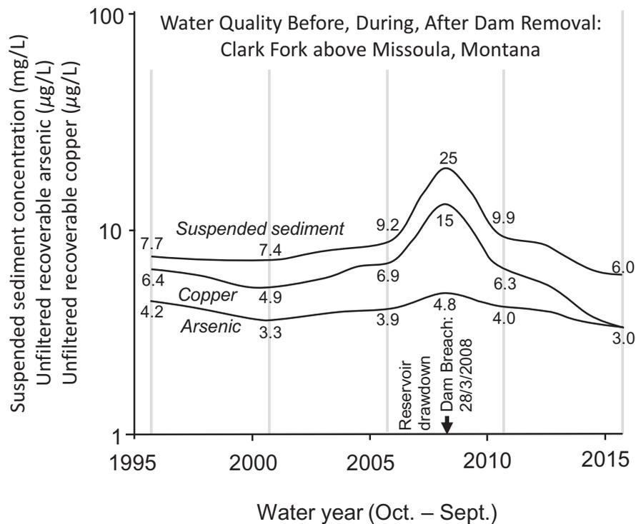
**Figure 4.39.** Arsenic, copper, and suspended sediment between 1996 and 2015 for Clark Fork River. Sampling was 4.8 km downstream of Milltown Dam. Note: y-axis is logarithmic (USGS station i.d.: 12340500). (Source: Sando and Vecchia, 2016.)
