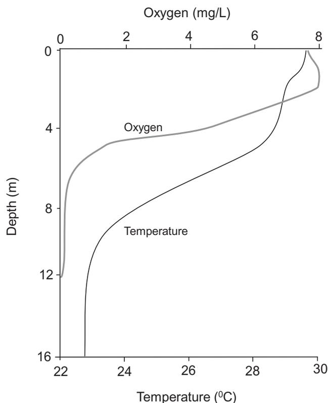
**Figure 4.33.** Reservoir depth (m) profile for water temperature (°C) and dissolved oxygen (mg/L) in 2004 for stratified Nam Leuk Reservoir, Laos, Mekong basin. (Source: Hortle and Nam, 2017.)
