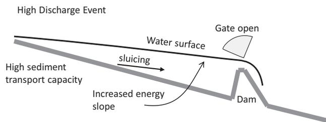
Figure 4.48. Profile of dam and reservoir operation during a sediment sluicing event, with gate opening timed with flood pulse. (Source: Kondolf et al., 2014a.)
