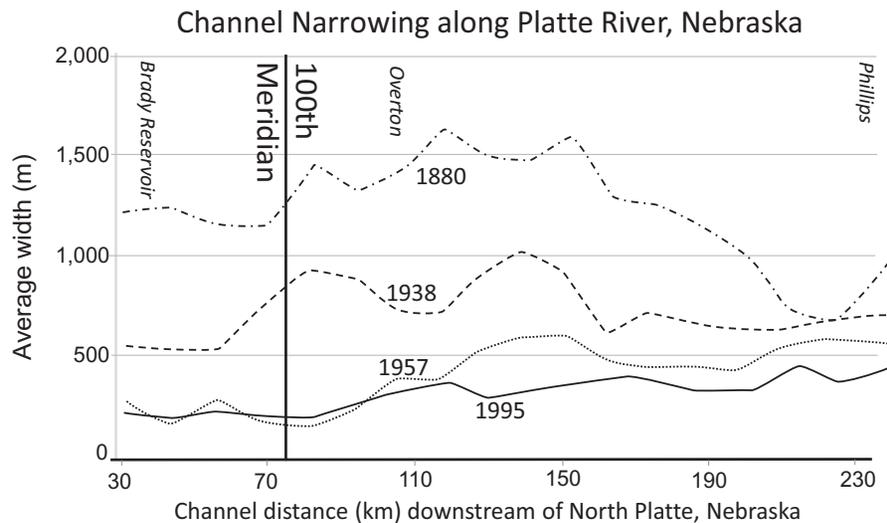
**Figure 4.28.** Changes to average channel width (m) along Platte River between Brady and Phillips, NE between 1880 and 1995. Kingsley dam is 118 km upstream of Brady Reservoir. (Source: Schumm, 2007.)
