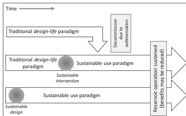
**Figure 4.53.** Models of dam and reservoir design related to sediment management. Conventional “design-life” paradigm for dams and reservoirs can be modified toward a sustainable use paradigm. New dam construction should include features adaptable to changing sediment management strategies. (Source: Annandale et al., 2016.)
