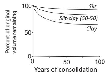
**Figure 4.40.** Reservoir sediment compaction over time for different particle size classes over one hundred years. Values are for continuously submerged deposits. Sand not shown because of minimal consolidation. (Source: Annandale et al., 2016.)
