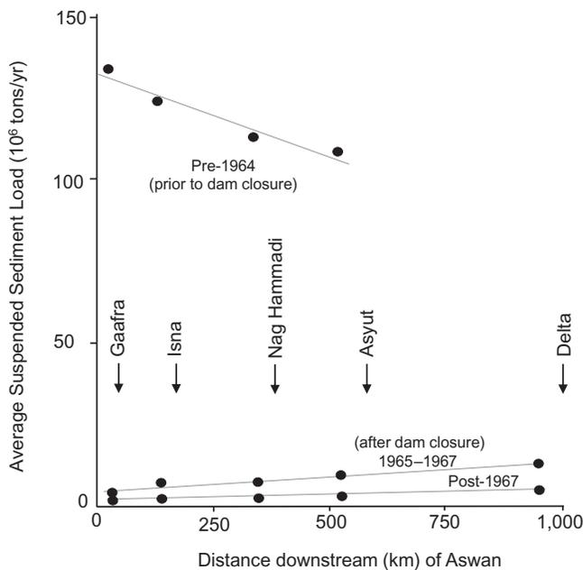
**Figure 4.16.** Downstream changes to suspended sediment loads along the Nile River before and after closure of Aswan High Dam in 1964. Suspended sediment comprises 30% clay, 40% silt, and 30% fine sand (Ahmed and Ismail, 2008). (Source: Morris and Fan, 1998.)
