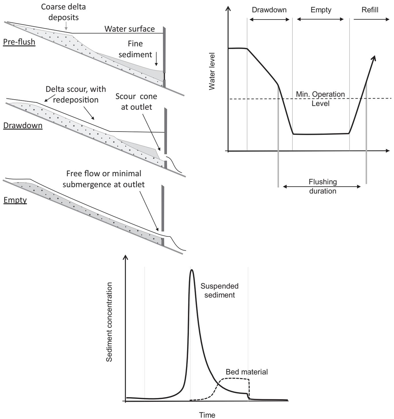
**Figure 4.50.** Profile of dam and reservoir operation during a sediment flushing event. Note drawdown occurs until reservoir is empty, which scours both fine-grained and coarser-grained reservoir deposits. High suspended sediment peaks occur prior to bed material mobilization. (Source: Morris, 2020.)
