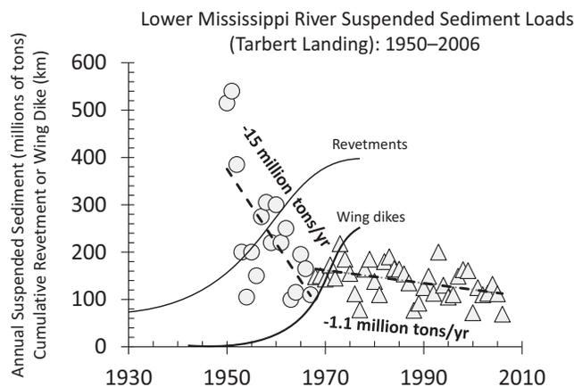
**Figure 4.24.** Historic change to suspended sediment loads for the lower Mississippi River at Tarbert Landing, Louisiana. Trend lines coincide with years 1950–1967 (–15 million tons/yr) and 1968–2006 (–1.1 million tons/yr). Cumulative distance (km) for revetment and wing dike (groynes) construction included for USACE Memphis and Vicksburg Districts. (Source: Meade and Moody, 2010.)
