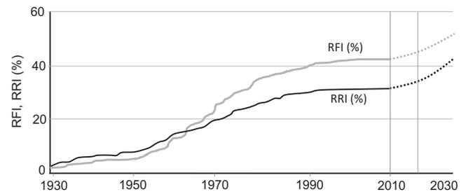
**Figure 4.10.** Global trend and future trajectory (to 2030) for the river fragmentation index (RFI) and river regulation index (RRI). Indices derived between 1930 and 2010 and estimated until 2030 (based on GRanD) for hydropower scenarios (dotted lines). Values reflect area-weighted means of indices across all basins. (Source: Grill et al., 2015, with data from Zarfl et al., 2015.)
