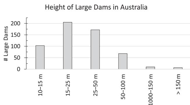
Figure 4.7. Large dams in Australia organized by height (m). Large dams in Australia are >15 m, or >10 m if reservoir >1,000,000 m<sup>3</sup> and maximum discharge >2,000 m<sup>3</sup>/s. (Data: ANCOLD, 2020.)
