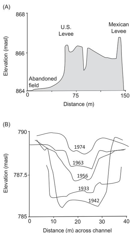
**Figure 4.27.** Changes to Rio Grande/Bravo at Presidio, Texas/Ojinaga, Chihuahua. (A) Deposition between the levees (dikes) resulting in embanked floodplain aggradation. (B) +3 m of channel bed aggradation and narrowing due to reduced flow conveyance caused by upstream impoundment and water withdrawal. (Source: Collier et al., 1996, data from Everitt, 1993.)
