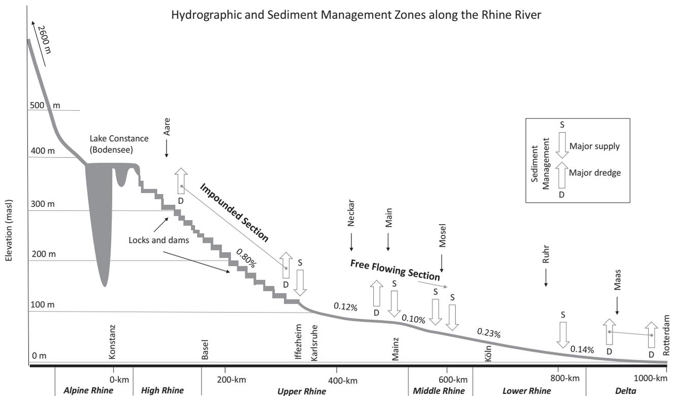
**Figure 4.20.** Longitudinal profile of the Rhine River, including geomorphic province, major tributaries, and sediment management operations. The stair-step pattern in the Upper and High Rhine is due to intensive impoundment. Gamsheim hydroelectric dam is located at 309-km, 25 km upstream of Iffezheim dam. (After Götz, 2008 and Frings et al., 2019.)
