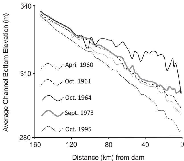
**Figure 4.51.** Longitudinal profile of reservoir deposits for Sanmenxia Dam, Huanghe River. Abrupt aggradation occurred soon after closure, and cessation of aggradation after effective reservoir management strategies implemented. (Source: Wang et al., 2005.)
