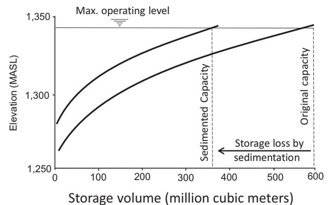
**Figure 4.46.** Reservoir elevation-storage: Comparison of original relationship and curve shift and storage volume lost due to reservoir sedimentation. (Source: Annandale et al., 2016.)
