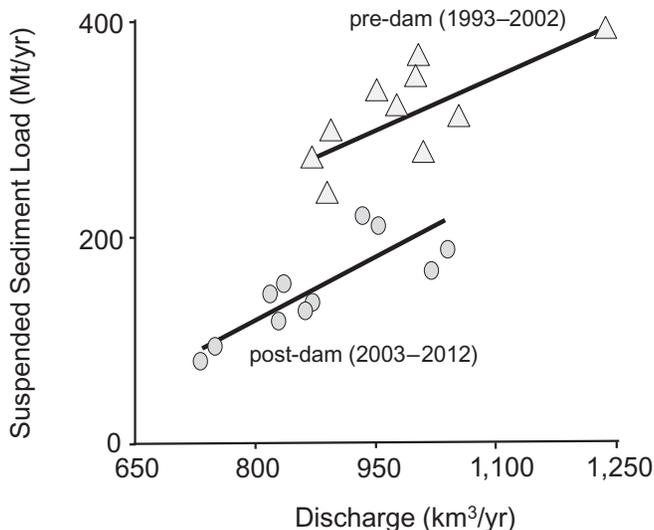
**Figure 4.17.** Comparison of annual discharge and suspended sediment loads before and after impoundment of the Yangtze River by Three Gorges Dam: Pre-dam (1993–2002) and post-dam (2003–2012). Datong is 565 km upstream of the river mouth. (Source: Yang et al., 2015.)
