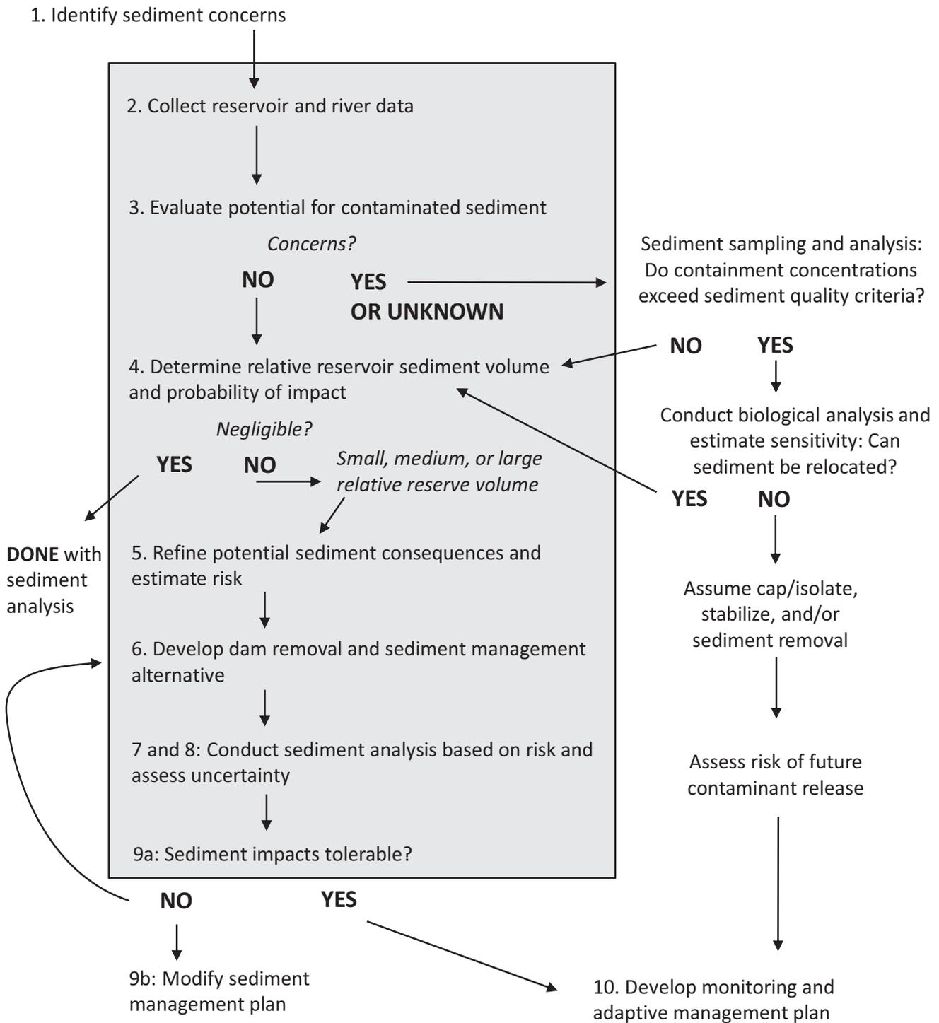
**Figure 4.38.** Steps for removal of reservoir sedimentary deposits. Sequence largely depends upon environmental concerns related to reservoir deposits. (Source: Randle et al., 2019.)
