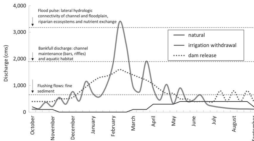
**Figure 4.11.** Conceptual model of annual flow regime for natural and impounded rivers, including “sawtooth” pattern from storage and release schedule for hydropower generation as well as withdrawal for irrigation to support agriculture during dry periods. (Author figure.)
