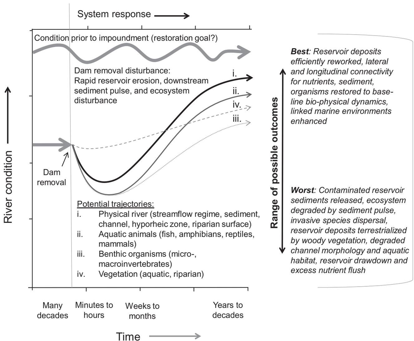
**Figure 4.44.** Conceptual model of river response to dam removal, including abiotic and biotic trajectories. The endpoints of possible outcomes, “best” and “worst,” range from full recovery of riverine geodiversity (physical integrity) and biodiversity to a completely degraded and polluted river associated with contaminated sediment release and a sediment pulse that obliterates channel aquatic habitat. (Figure developed after Foley et al., 2017; Doyle et al., 2003b; and others.)
