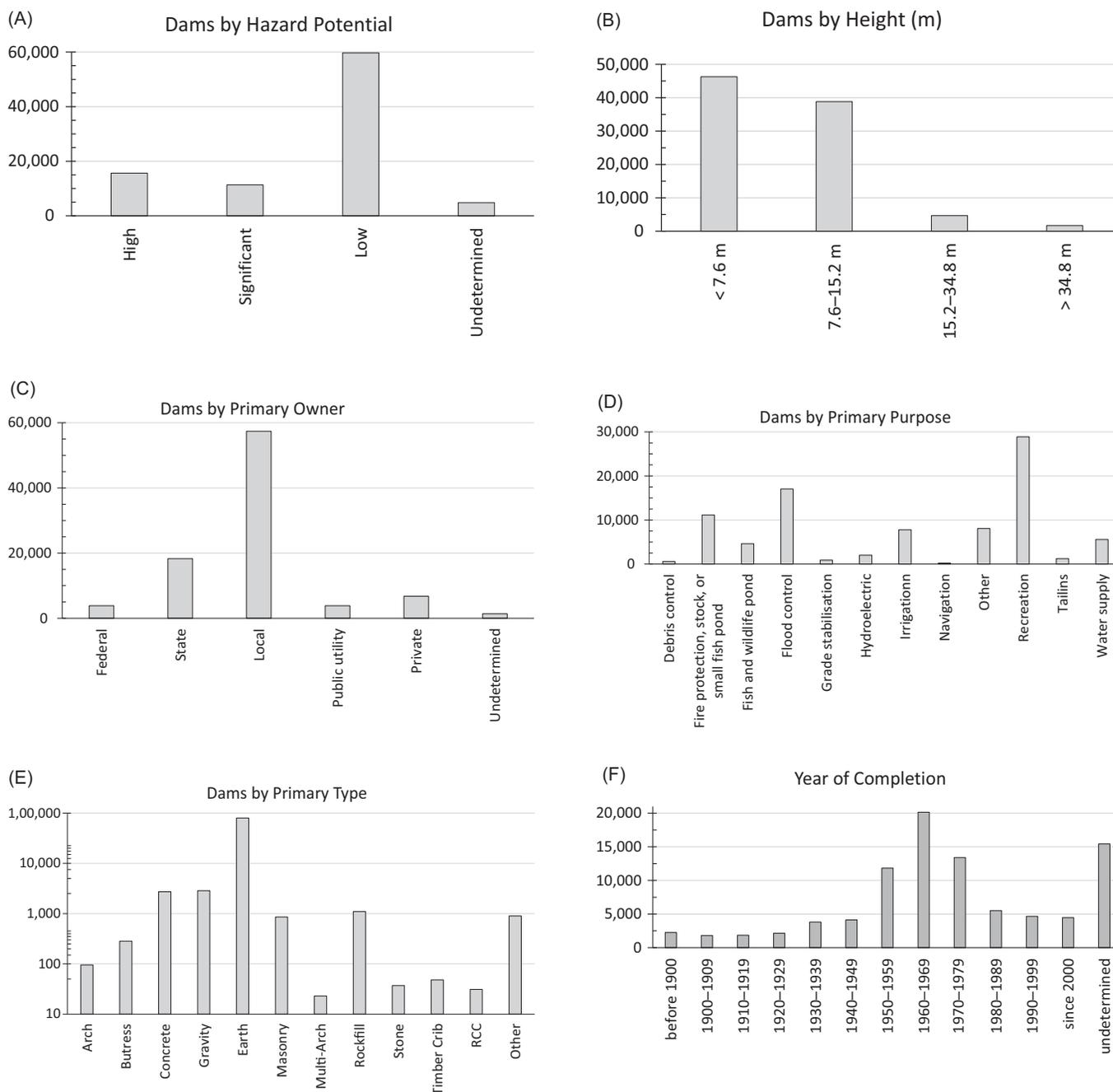
**Figure 4.8.** The United States has 91,457 dams (A) decade of completion, (B) height, (C) primary purpose, (D) primary owner, (E) primary type, and (F) hazard potential. Note: y-axis for dam type (E) is logarithmic. (Author figure. Data source: U.S. Army Corps of Engineers National Inventory of Dams.)
