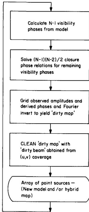
Fig. 1. Flow diagram for a linear reconstruction method using closure phase
