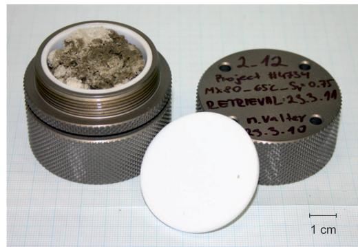
FIG. 2. Containers (ematal aluminium with inner PTFE casing) encapsulating granular MX-80 (dry bulk density 1.5 g/cm<sup>3</sup>) during thermal treatment. The inhomogeneous water distribution (saturation degree 75%) is visible. The dark granules had a higher water content.
