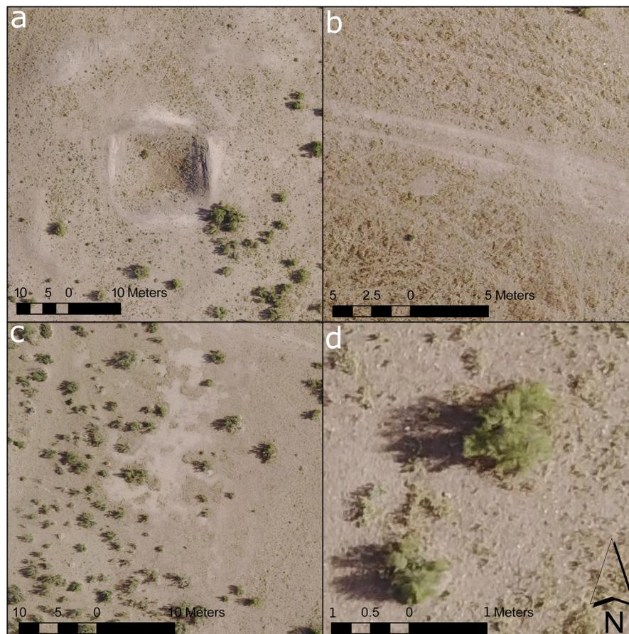
**FIGURE 6.** Details of topographic features identified in the models: (a) old excavation trenches and backfill, (b) tire tracks and livestock paths, (c) distinction between bare clay ground surface (*takyi*) and sand cover, and (d) individual bushes.
