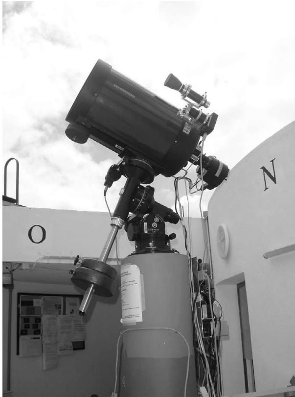
**Figure 1.** The 11" telescope in its mount at the main campus of INPE.
