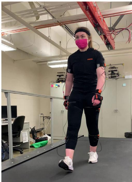
**Figure 1.** Subject wearing XSens inertial motion capture suit, making changes of intended walking speed on large research treadmill.
