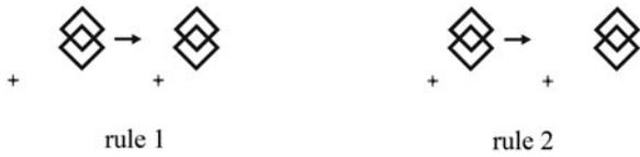
Fig. 15. Parametric rule 1 moves the added shape left. Parametric rule 2 moves it right.
