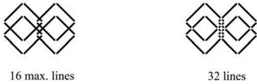
**Fig. 24.** The shape  $C_2$  includes 16 maximal lines (left). A discrete decomposition of 32 linear segments enables the recognition of all emergent squares (right).
