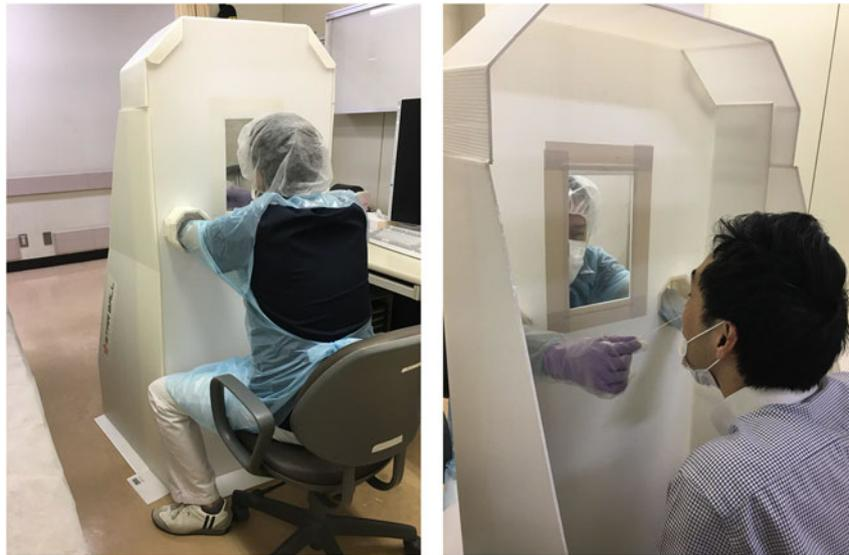
**Fig. 1.** The photo shows the healthcare worker (HCW) and patient sides of the shield. An acrylic plate is used for the window so that the patient's face can be seen clearly. The HCW wears PPE for examinations but does not need to change PPE for each patient. The disposable gloves used for testing must be changed for each patient.
