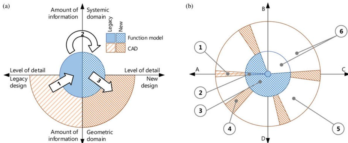
**Fig. 7.** Design space exploration process using FMs as an intermediate step. (a) Illustrates the steps (1) functional decomposition, (2) innovation, and (3) embodiment to get from legacy to novel design. (b) Provides a top view of the same graph, showing the design space (5) and how it can be explored using function (2, 3) and geometry (1, 4) models.
