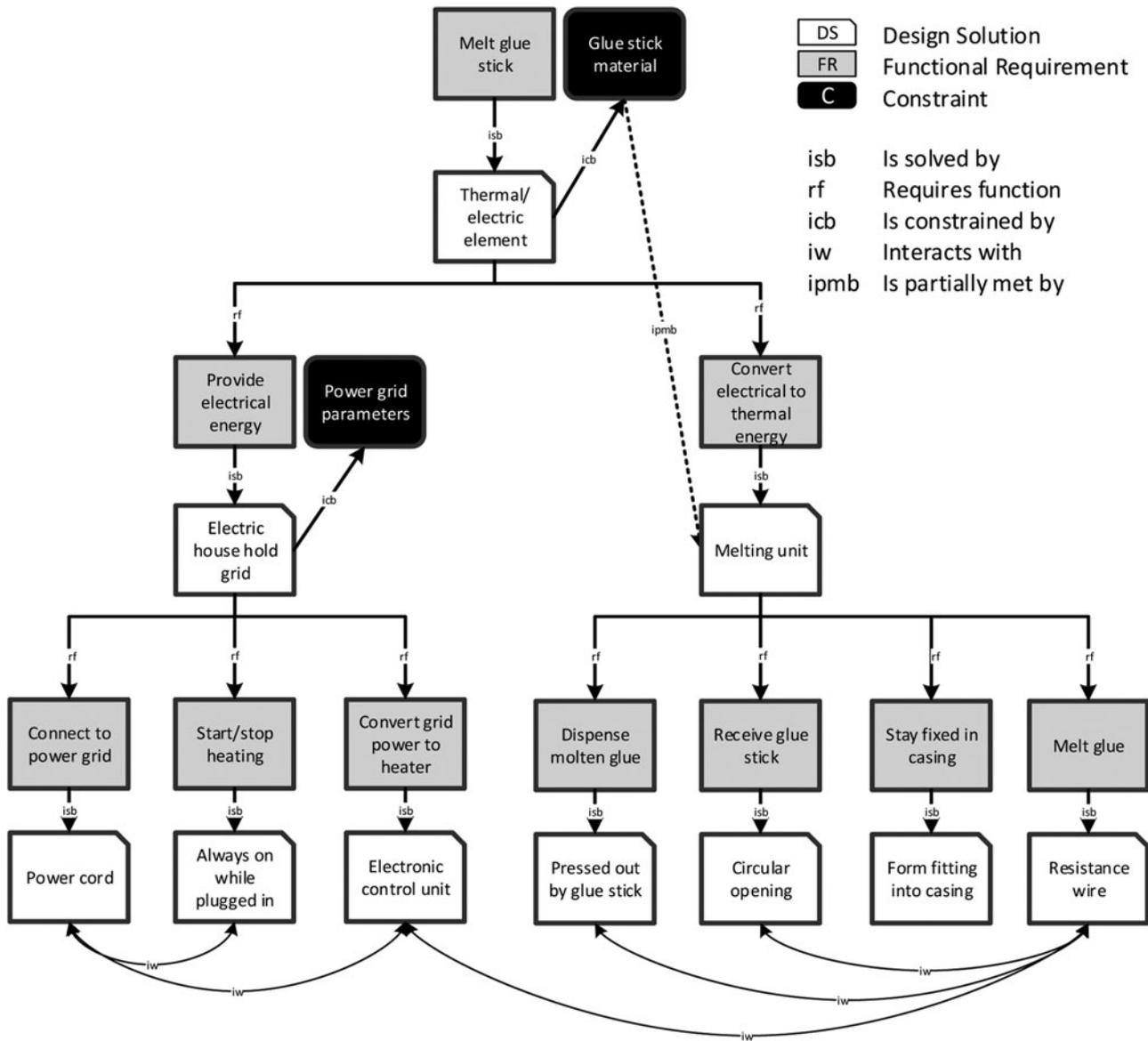
Fig. 3. Function decomposition of DS “Thermal/electric element”.
