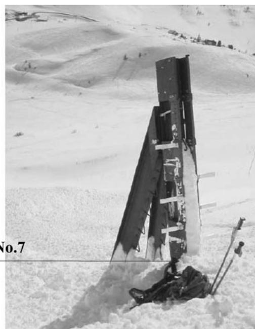
Fig. 5. Aluminium targets on wedge in path 2 at Lautaret avalanche site.
