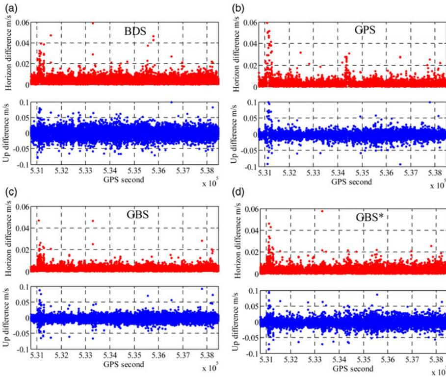
Figure 13. The 3D velocity difference between the stand alone velocity solution and the reference velocity.
