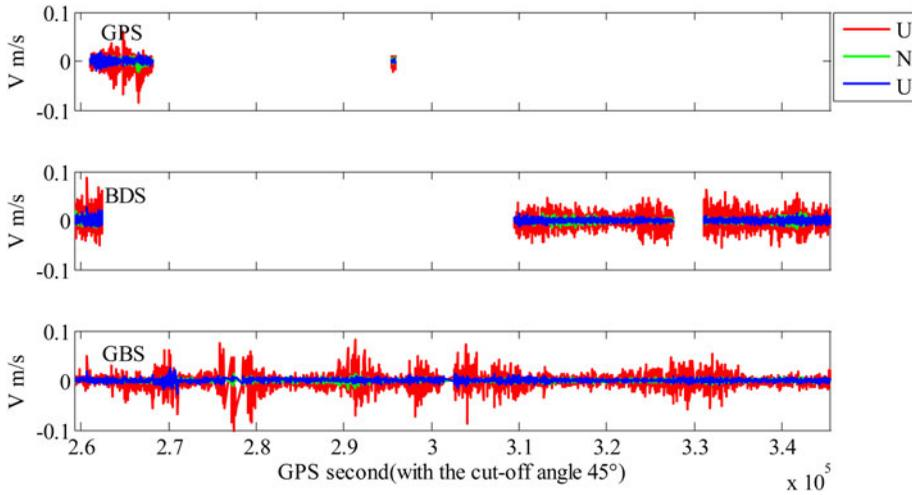
Figure 9. Scheme2 Velocity estimation using LC for East/North/Up components with the cut-off angle 45°(station: WHCD).
