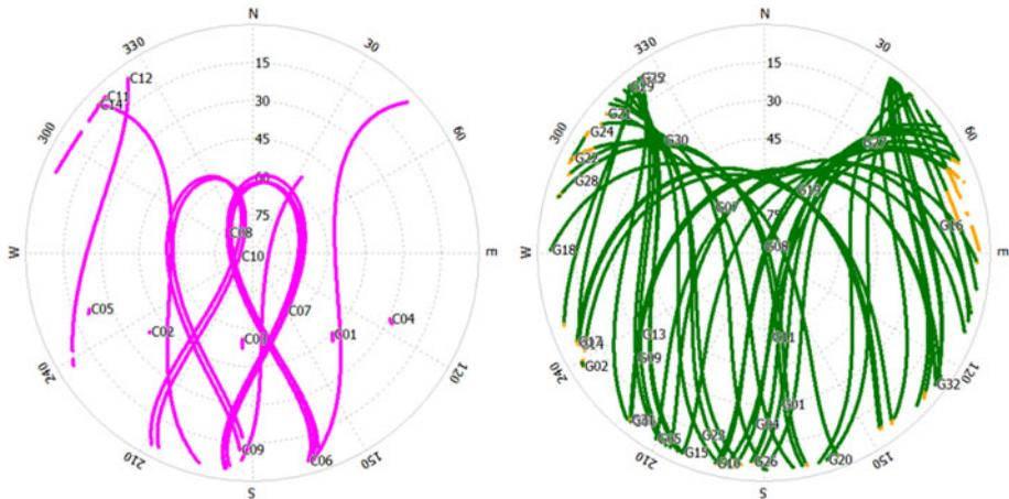
Figure 3. Sky plots of BDS (left) and GPS (right) satellites of station WHCD. The purple lines represent observations with B1/B2 frequencies, the green lines represent observations with L1/L2 frequencies, and the yellow lines represent observations with L1 frequency only.
