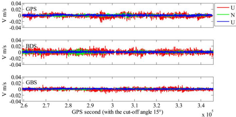
Figure 7. Scheme2 Velocity estimation using LC for East/North/Up components with cut-off angle 15°(station: WHCD).
