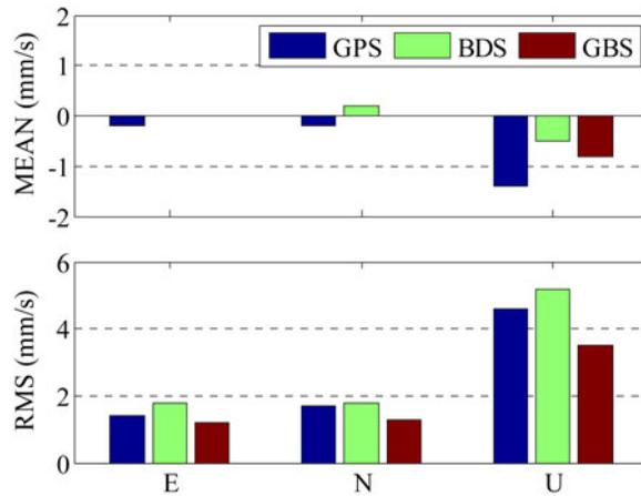
Figure 6. The precision statistics of velocity estimation for GPS, BDS and GPS/BDS using LC from 8 stations.
