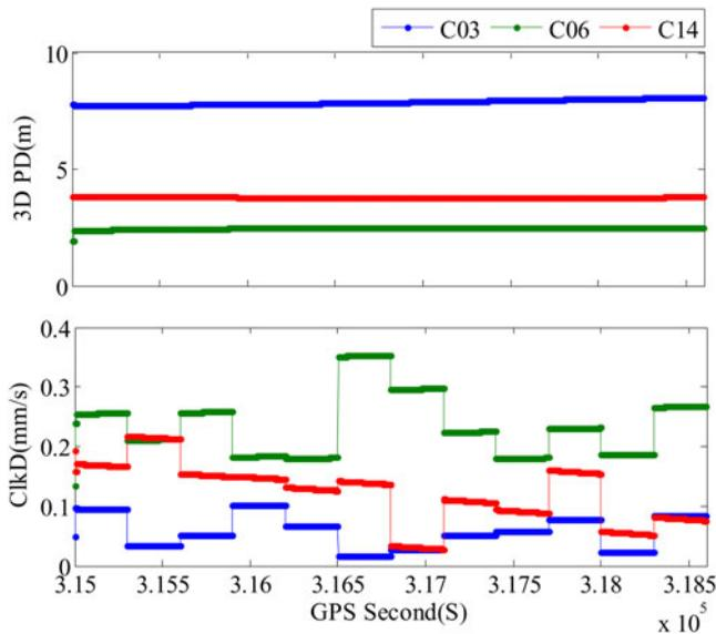
Figure 2. Proof that the satellite position and clock drift calculated by using the broadcast ephemeris is sufficiently accurate in comparison with SP3 precise ephemeris (PRN = C03/C06/C14,15:30:00~16:30:00, 10/01/2014).
