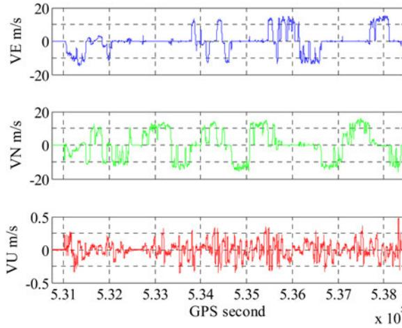
Figure 12. Velocity obtained from DGPS with first-order central difference of a Taylor series approximation. These three panels illustrate East, North and Up components of the velocity.
