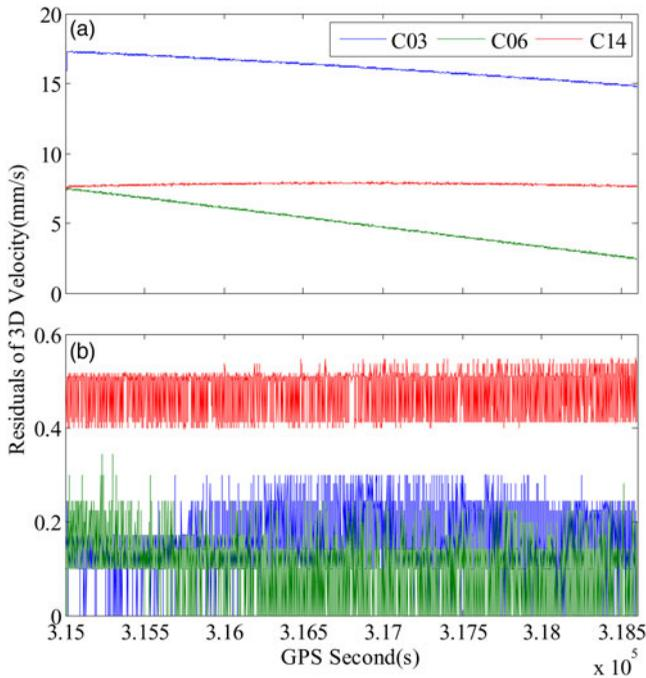
Figure 1. Residuals of satellite velocity obtained from the closed-form formula (a) and position-derivation (b) compared with the velocity obtained from the SP3 precise ephemeris using first-order central difference of a Taylor series approximation (PRN = C03/C06/C14,15:30:00~16:30:00, 10/01/2014).
