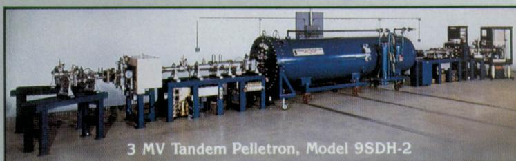
3 MV Tandem Pelletron, Model 9SDH-2
