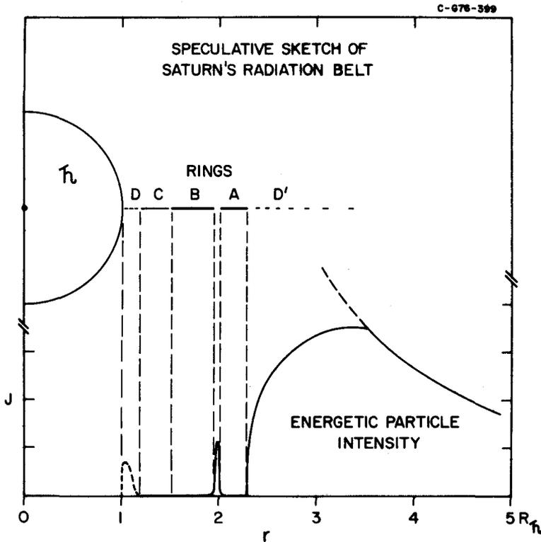
**Fig. 11.** The upper part of the diagram is a scale drawing of a meridional cross section of Saturn and its D, C, B, A, and D-prime rings of particulate matter. The lower part is a speculative sketch of the radial dependence of the intensity of energetic particles in its magnetosphere. The nature of the curve for  $r > 2.3 R_S$  is a sensitive measure of the opacity of the D-prime ring.
