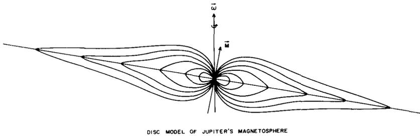
Fig. 8. Schematic drawing of the magnetodisc model of the outer magnetosphere of Jupiter, showing topology of the magnetic field and the region of trapped energetic particles. The outer tip of the sketch is at  $\approx 100 R_J$ . The planet's rotational axis is denoted by  $\vec{\omega}$  and its magnetic axis by  $\vec{M}$ .
