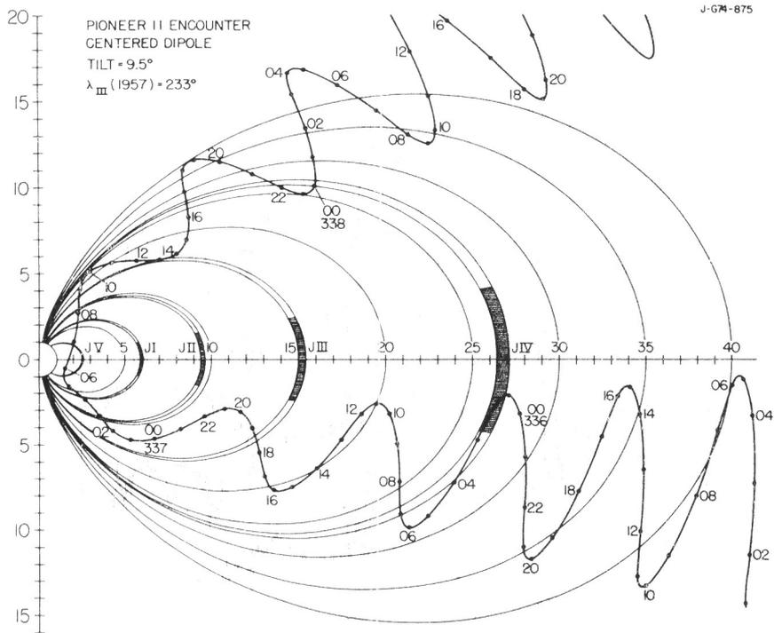
**Fig. 2.** Time-labeled trace of Pioneer 11's encounter trajectory on a magnetic meridian plane through the spacecraft. The assumed Jovian dipolar model is specified. The cross-hatching shows the regions that bound the orbits of JV (Amalthea), JI (Io), JII (Europa), JIII (Ganymede), and JIV (Callisto) in this coordinate system. The time is "Earth Received Time" as in Figure 1.
