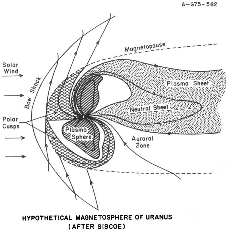
Fig. 14. Hypothetical physical structure of a Uranian magnetosphere during the epoch of pole-on presentation to the solar wind (Siscoe 1975).
