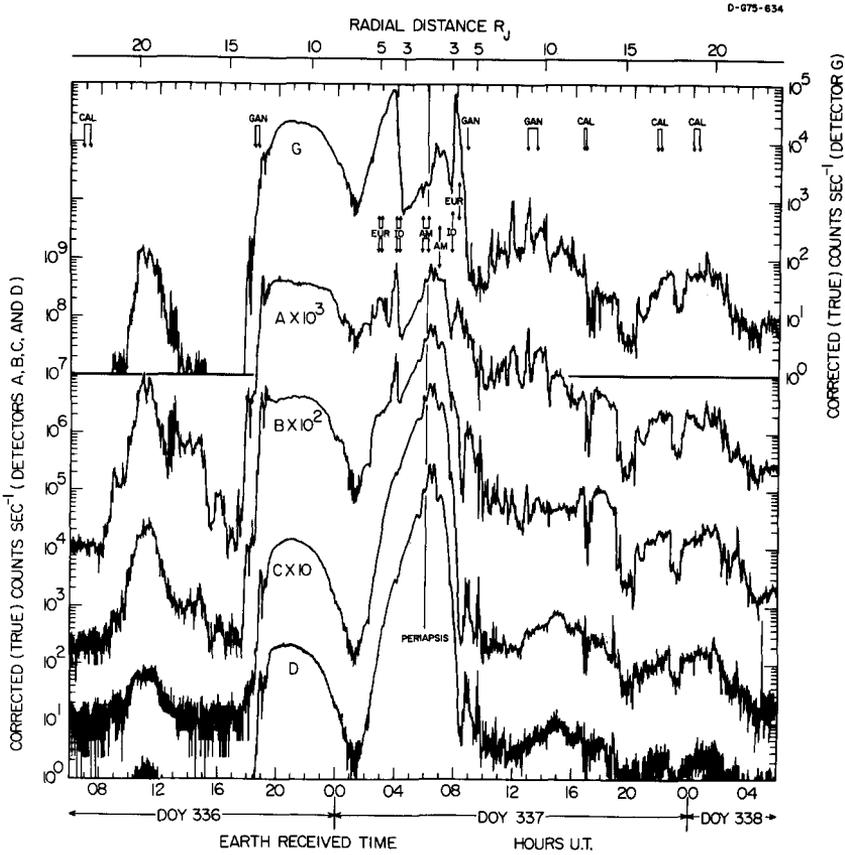
**Fig. 3.** Time dependence of the corrected, spin averaged counting rates of five particle detectors (cf. Table I) during a portion of the encounter with Jupiter. The times of traversal of nominal dipolar magnetic shells of the five inner satellites are shown by vertical arrows. These times may be appreciably in error for JII, JIII, and especially JIV by virtue of distortion of the magnetic field from dipolar form. DOY means day of year. The year is 1974.
