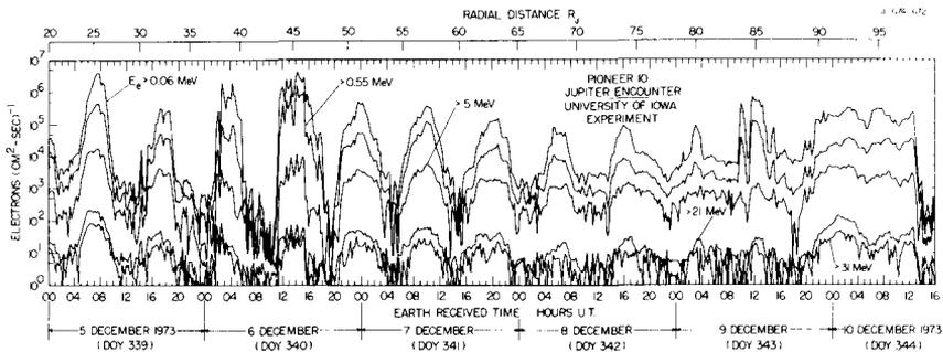
Fig. 7. Time dependences of the omnidirectional intensities of electrons in five different energy ranges during the Pioneer 10 outbound traversal of the outer magnetosphere on the dawn side of the planet.
