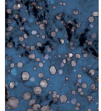
Radiation-induced defects such as voids restrict materials choices for fourth-generation reactors.
