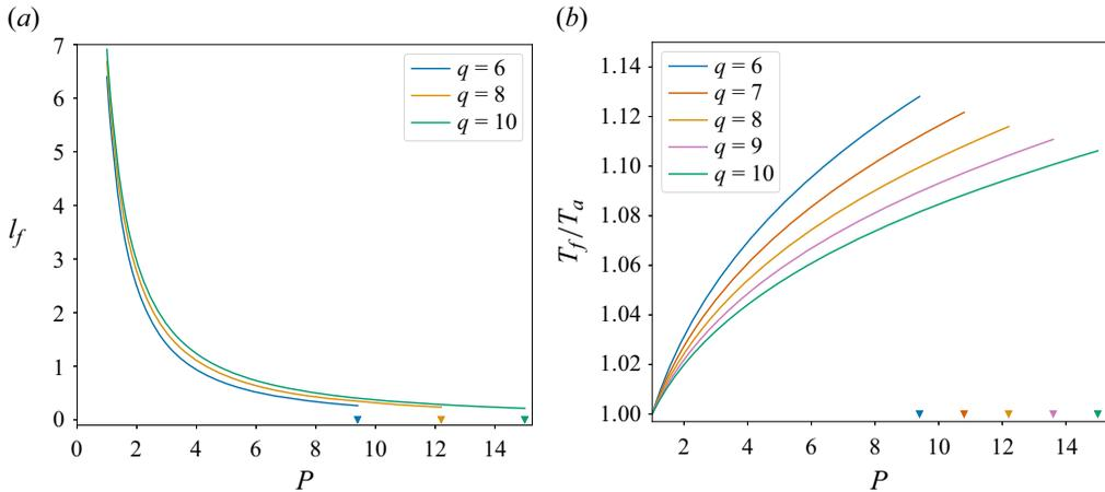
Figure 2. The dependence of (a) the flame thickness  $l_f$  and (b) the flame temperature  $T_f$  scaled by the adiabatic flame temperature  $T_a$  on pressure  $P(t)$  representing time, for various values of the heat release parameter  $q$ ; the curves end at  $P = P_e$  marked on the axis.
