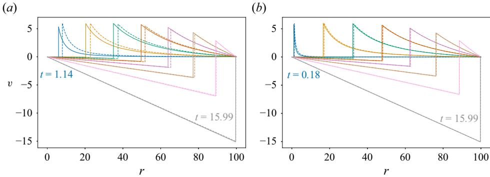
Figure 12. Velocity profiles of a spherical flame propagating in a closed vessel at equal time intervals. The dashed lines correspond to the leading-order solution, absent of stretch effects, and the solid lines to the solution with  $O(\delta)$  contributions included; for  $q = 6$  and  $Le_{eff} = 1$ . Results are shown for (a)  $\delta = 0.05$  and (b)  $\delta = 0.001$ .
