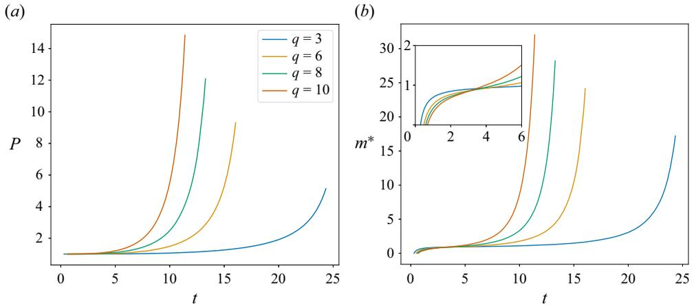
Figure 10. The pressure  $P$  and burning rate  $m^*$  as a function of time, for a spherically expanding flame in a closed vessel at various values of the heat release parameter  $q$  and  $Le_{eff} = 1$ .
