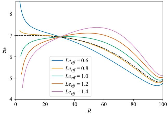
Figure 14. Propagation speed of spherical flames for various  $Le_{eff}$ ; plots correspond to  $q = 6$  and  $\delta = 0.05$ ; the dashed line indicates the solution (leading-order) in the absence of stretch effects.
