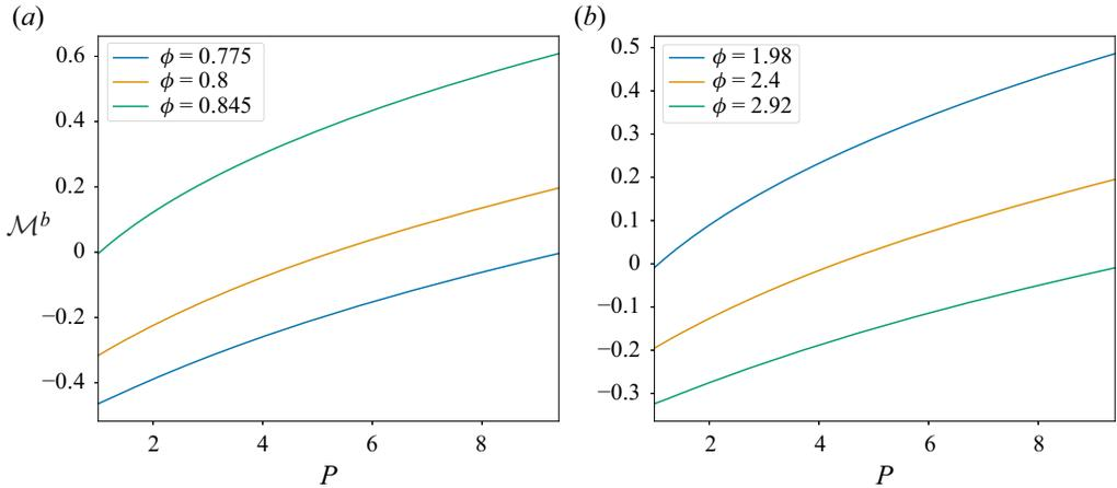
Figure 5. Two cases illustrating circumstances where the ‘burned’ Markstein number  $\mathcal{M}^b$  may change sign during the propagation. Results are shown for the (a)  $\text{H}_2$ -air mixture and (b)  $\text{C}_8\text{H}_{18}$ -air- $\text{CO}_2$  mixture.
