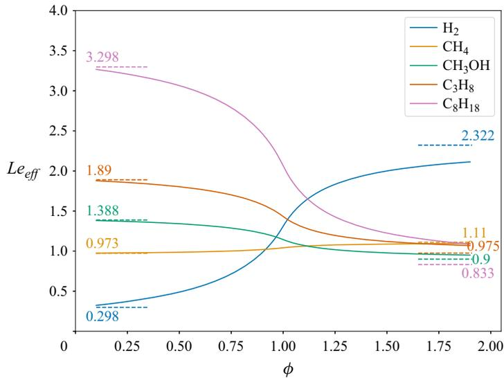
Figure 3. The dependence of the effective Lewis number  $Le_{eff}$ , averaged over the total propagation time, on the mixture equivalence ratio for several fuels burning in air. The dashed lines mark the limiting Lewis numbers; the fuel Lewis number  $Le_F$  for lean mixtures and the oxygen Lewis number  $Le_O$  for rich mixtures.
