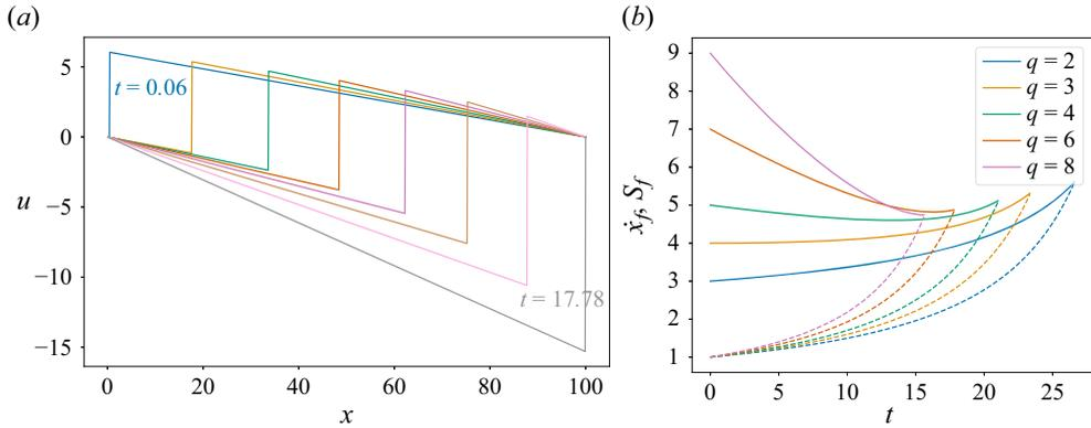
Figure 9. Planar flames propagating in a closed channel: (a) velocity profiles at equal time intervals, for a representative value  $q = 6$ , and (b) flame speed  $S_f$  (dashed curves) and propagation speed  $\dot{x}_f$  (solid curves) as a function of time for various values of  $q$ .
