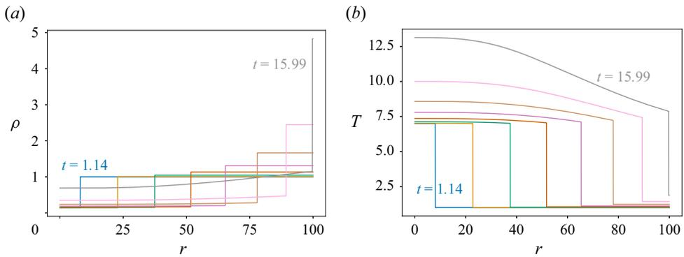
Figure 11. Density and temperature profiles of a spherical flame in a closed vessel at equal time intervals, for a representative value  $q = 6$ .
