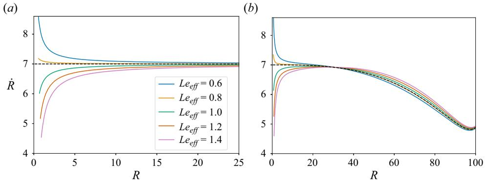
Figure 13. Propagation speed of spherical flames for various  $Le_{eff}$ ; plots correspond to  $q = 6$  and  $\delta = 0.001$ ; the dashed line indicates the solution (leading-order) in the absence of stretch effects. (a) Freely propagating flame. (b) Propagation in a closed vessel.
