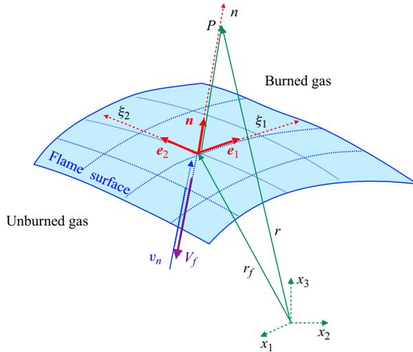
Figure 1. The intrinsic curvilinear coordinates  $(\xi_1, \xi_2, n)$  to the flame surface. The blue and magenta vectors correspond to the normal component of the gas velocity  $v_n \mathbf{n}$  and normal propagation velocity  $-V_f \mathbf{n}$ , respectively.
