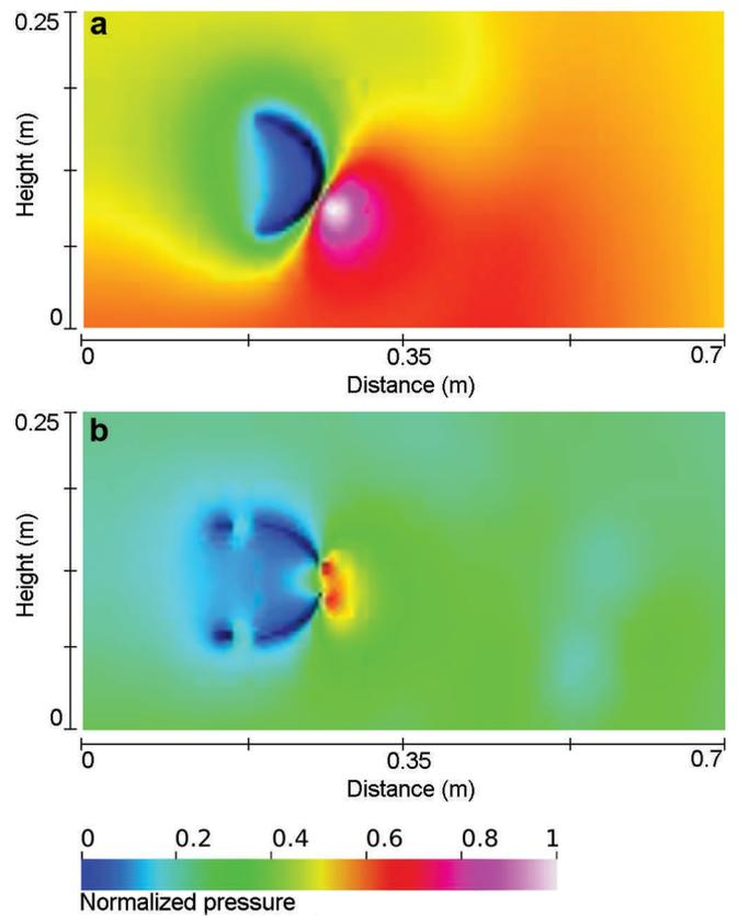
**Fig. 7.** Results of finite-element modelling the aerodynamics of components of ADIOS. Normalized air pressure around (a) a solid flat circular parachute and (b) a Disk Gap Band parachute. The direction of airflow was left to right.
