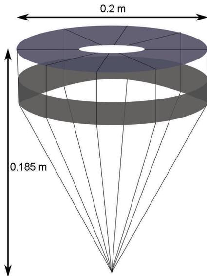
**Fig. 6.** Disk Gap Band parachute design.
