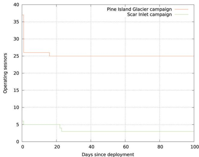
**Fig. 11.** Lifetime of the 43 ADIOS-GPS sensors on Pine Island Glacier and Scar Inlet.
