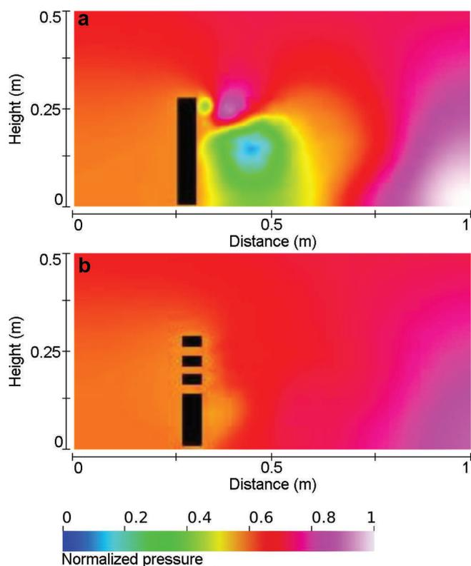
**Fig. 4.** Results of finite-element modelling the aerodynamics of components of ADIOS. Normalized air pressure around (a) a solid snow brake and (b) a geometrically porous snow brake. The direction of airflow was left to right.
